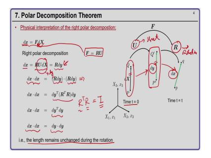
So, we know that d x dot d x that would be nothing, but. So, I mean sorry we want to show that the length of vector d y is same as the length of vector d x ok; because that is where rotation is involved. So, we start with the scalar product of the spatial vector d x dot d x and now d x is nothing but R dy d x is R d y; so substituting that we get R d y dot with R d y ok.
