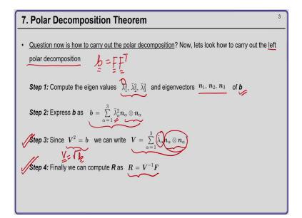
So, that is what we want to do today left polar decomposition. So, we will start with the left Cauchy Green tensor which is given by F F transpose. Now, you have been given the deformation gradient tensor F and now you can compute b. So, the steps to carry out the polar decomposition remains same as discussed previously ok; when we saw how to do polar decomposition using right polar decomposition theorem ok.
