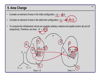
Coming to the final point: So, the final point now is how do we relate the areas in the initial and the final configuration? So, consider again this body the initial configuration is B 0 bounded by surface del B 0 which after deformation we have in the final configuration B bounded by surface del B.
