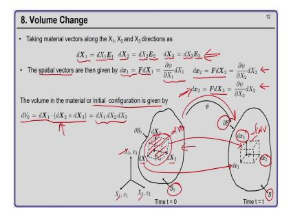
So, first we look into the volume integral. So, the picture here shows; the body at time 0 in that is in the integral configuration and let us say you have this volume. So, at point P you have this infinitesimal volume d V and you have material vectors d X 1, d X 2, d X 3 which are aligned along the X 1 X 2 and X 3 directions respectively. So, in a finite element setting this dotted lines would actually refer to the one particular finite element ok.
