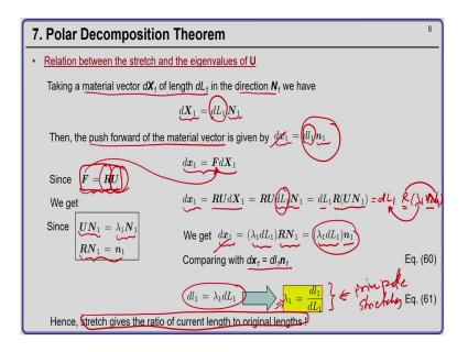
So, we can substitute U N 1 as lambda 1 N 1. So, we can substitute U N 1 as lambda 1 N 1. And now once we have lambda 1 N 1 here we will have d L1 R lambda 1 N 1 capital N because lambda 1 is a scalar I can take on this side. So, we are left with R times N 1. So, R N 1 is nothing, but small n 1 ok. So, using this we will get the spatial vector d x 1 as lambda 1 d L 1 equal to R N 1 which is nothing, but lambda 1 dl 1 equal to lambda 1 d L into n1 ok.
