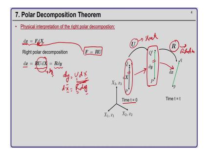
Now, we move to get a physical interpretation of right polar decomposition. So, deformation gradient tensor F maps the material vector d X to the spatial vector d small x that we know. Now, the polar decomposition right polar decomposition gives you F equal to R into U. Therefore, if you substitute for F here if you substitute for F here we will get the spatial vector d x equal to R U times d capital X the material vector d X ok.
