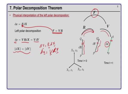
So, in left polar decomposition we have F equal to V R. So, substituting this here so the spatial vector is nothing but V R d X, which is nothing but V d Y d capital Y. So, how can we interpret this? Ok, so first there is only rotation because d Y is sorry this a vector. So, one under bar R d X ok.
