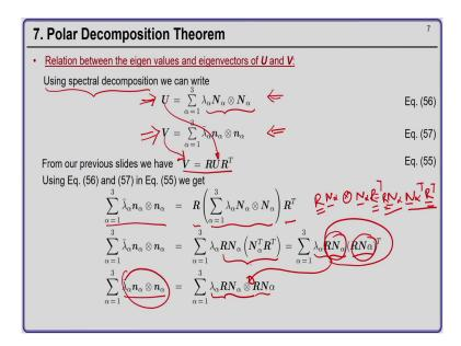
So, now next is we want to have a relationship between the eigenvalues and eigenvectors of the right and the left stretch tensors. So, recall from our previous discussions that using spectral decomposition we can write the right stretch tensor in terms of its eigenvalues and eigenvectors given by equation 56 ok. In similar manner we can write the left stretch tensor in terms of its eigenvalues and eigenvectors which is given the equation 57 ok.
