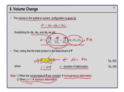
Now, similarly I can write the volume in the spatial on the or the current configuration as d V equal to d x 1 d x 2 cross d x 3. Now, I can substitute for d x 1 d x 2 d x 3 from the previous slides we have those expressions and I can write d V as del sorry this is del psi by del X 1 dot del psi by del X 2 del cross del psi by del X 3 into d X 1 d X 2 d X 3 ok.
