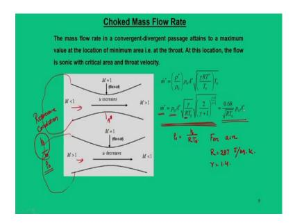
So, by putting this expressions; we can arrive at a working formula which is known as, mass flow rate in the convergent divergent passage and that attains to a maximum value at the minimum area location; that is throat. So, when I put this expression and finally, after simplification we arrived at this particular relations.
