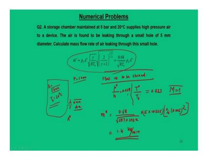
The another simple problem that talks about a storage chamber is to be maintained at 5 bar and 20°C; that supplies high pressure air to a device. The air is found to be leaking through a hole of 5 mm diameter. Calculate the mass flow rate of air leaking through the small hole.
