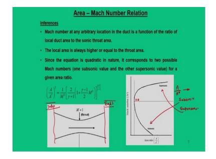
So, here what we see that for a given area ratio, there are two possibilities; one is in the subsonic, other is in supersonic. So, the subsonic solution goes to the bottom part of the curve, supersonic solution goes for the top part of the curve.
