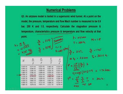
The third problem which I am talking about is that; how to refer a gas table? So, what has been given that an airplane model is to be tested in a supersonic wind tunnel where at any point in the model, the pressure is given as 0.9 bar, temperature is given as 250 Kelvin, Mach number is given as 1.5.
