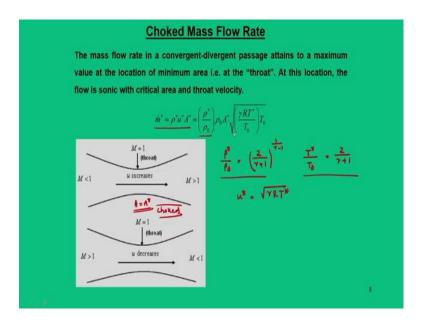
Now, the another important segment of this convergent divergent passage is the choked conditions. The choked condition is essentially decided by the fact that the flow is sonic at the minimum area. So, when the flow is sonic at this minimum area, that is  $A = A^*$ ; then we say it is a choked condition. So, when I say choked condition, this is possible for whether your inflow is subsonic or whether the inflow is supersonic.
