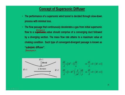
The reverse situation that occurs that means, in most of the wind tunnel applications, when you first we increase the flow to a supersonic value, but we must slow down the process with minimal loss; that means, when we release that gas to the exit atmosphere, it should be such that it should encounter minimum loss. So, to have this minimum loss, we cannot dump that high speed air just like into the atmosphere.
