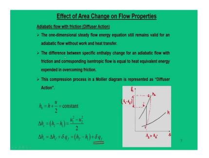
Now, in similar concept also apply here, but here the heat equivalent energy expended in overcoming friction for the situation of a diffuser action happens to be a positive quantity. So, in the same plot h-s, one can say that I am at  $p_1$ , I am moving to  $p_2$ . So, here an isentropic process would have gone to 1 to 2; but a non-isentropic process will take to a real situation and your  $h_2$  also greater than  $h_2$ .
