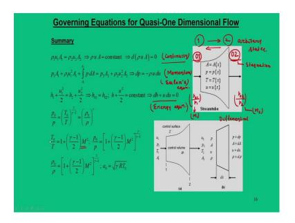
So, just to summarize whatever you have studied, I can make out that we are looking a quasi one dimensional flow approach where the area can change; but this area can change in a particular direction that is A as a function of x. It is first approach, first assumption of quasi one dimensional flow, essentially the flow is one dimensional; but it is still not one dimensional, but we are relaxing the dimensionality in some aspect. So, we say it is a quasi.
