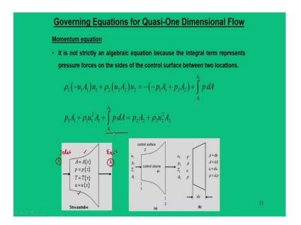
Now, moving to the momentum equations; momentum equations essentially it is a not strictly a algebraic equations, because the area change matters. So, what we see is that, from inlet to exit that is from 1 to 2 what we see is that the area that comes by virtue of pressure is  $p_1A_1$  that is for this side and area that comes by virtue of exit is that  $p_2A_2$ . The press force that get exerted on this exit area is  $p_2A_2$ .
