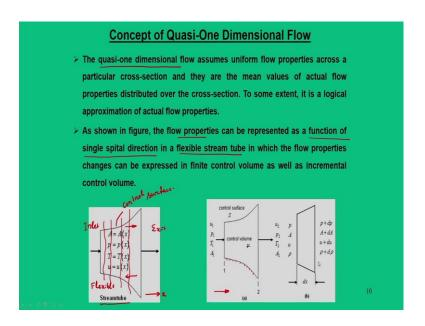
So, you bring this particular concept here is that, this is a kind of a situation where we can say the; it is a kind of a duct which has certain inlet area  $A_1$  and also some exit area  $A_2$  and in this case the area changing only in the direction of x. So, I can write A as a
