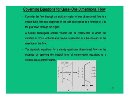
So, these are already I have explained, just to go through these, just I can just read out that; we are now moving for quasi one dimensional flow analysis for which we are going to derive the governing equations. In this case, we are we have to consider any arbitrary region in the one dimensional flow through a stream tube. The flow properties in the tube can change as a function of x.
