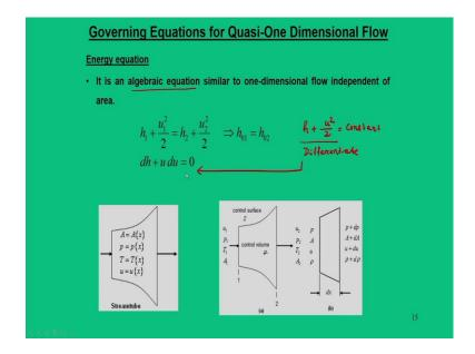
Now, moving to the energy equations; now as you can see the energy equation is still algebraic, because the flow is isentropic. So, total enthalpy remains constant, that is  $h_{01} = h_{02}$ . And, when I say total enthalpy is remains constant; that is if I write  $h + \frac{u^2}{2} = const$  and differentiate this equation, then we move to the equation that is dh + udu = 0.
