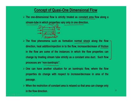
So, in a quasi one dimensional approach what really happens is that, in a normal situation we say the flow to be one dimensional contained infinite number of streamlines and we assume this to be a stream tube. And we are really bothered about the inlet and exit conditions, that is 1 and 2 and we say this process needs to be isentropic.
