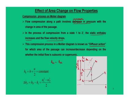
Now, moving further we will just take a reverse situation. So, there is nothing just to explain here we are just saying that, it is a compression process on a Mollier diagrams. So, we redraw the same figure. So, I will just put the reverse symbol like we are now at point 1 and moving to point 2 that is pressure must increase; but still your stagnation pressure remains same.
