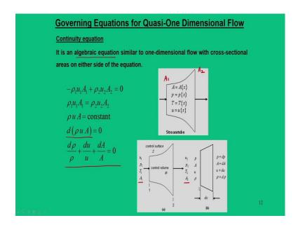
So, the first equation that comes out is the continuity equation; so obviously the continuity equation is a straight forward, its a algebraic equations, the very basic difference what we are bringing here. Whereas in previous equations, where the area was assumed to be constant; but here we are saying area as  $A_1$  that is section 1 and area as  $A_2$  here.
