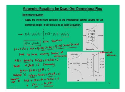
And what we are trying to look at here, we have to revisit the concept that we are dividing this entire control volume with small elemental length dx or elemental area dA and area changes from A to A+dA. So, accordingly when the area changes this; so the thermodynamic properties pressure, velocity and density they also change in a very small manner like p+dp, u+du and  $\rho$ +d $\rho$ .
