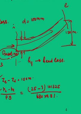
The next problem talks about the use of what I can say Bernoulli's equation or in other words we can rewrite as steady flow energy equation that involves head loss. So, when there is no head loss this steady flow equation turns out to be Bernoulli's equation.
