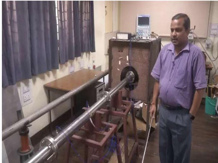
So, now let us move to the instrumentation side for the driven sections. So, we have seen that when the shock wave propagates in the driven section, across the shock wave there is an instantaneous rise in pressure of the induced mass. So, to measure that step response of this induced mass pressure, we have mounted two pressure transducers and one is at this location which is 1885 millimeter from the end planes.
