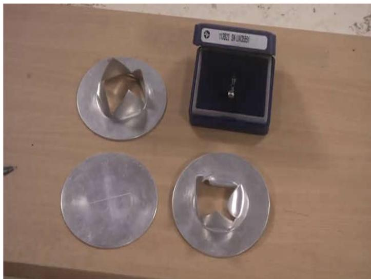
So, we are going to show now that how a diaphragm looks like before before its rupture and after its rupture. So, what we see here is the first diaphragm and for this first
