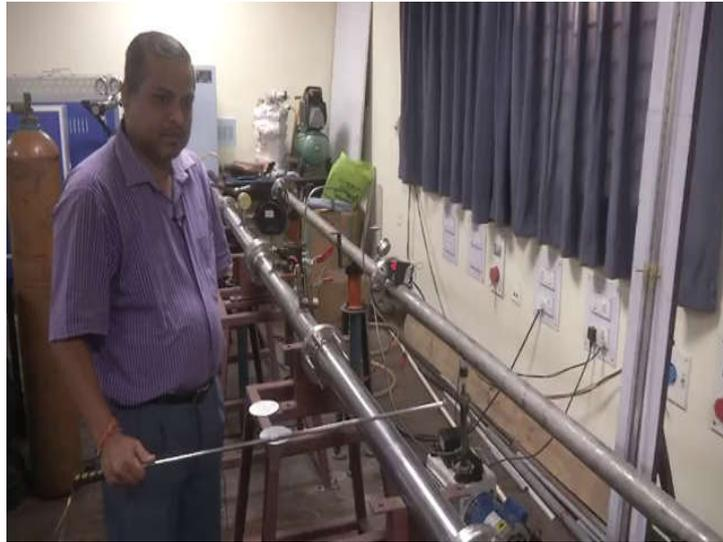
Now, we are moving to the driven section of the tube. So, driven section of the tube is of similar length and material as used in the driver sections. So, as a thumb rule when we are using two tubes of driver section of 1 meter length, similarly we have to use minimum of 5 meter of driven section length.
