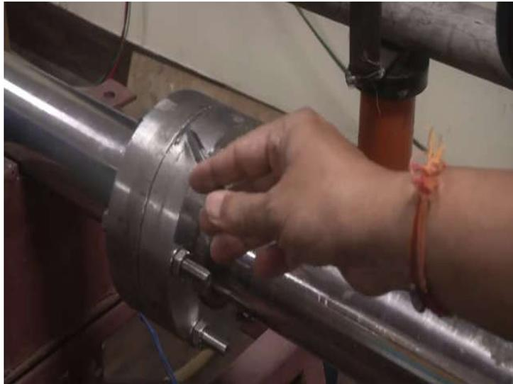
So, as you see that to have inserted a diaphragm at this interface location between driver section and driven sections, and this pressure of the driver section we are going to record in a pressure gauge.
