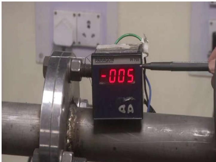
So, for this pressure gauge you can see there is a reference line which is almost 0, but; however, this is the instrument bias error, there is a marginal error. However, we can put this as a reference line which is seen that there is a almost the pressure or what you say with respect to this value is 0.
