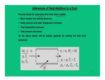
So, from this equations one can talk about two important informations; one is what happens if your upstream condition is a supersonic flow, when heat is added. In fact, there are four possibilities; the first two possibilities could be inflow can be supersonic or subsonic and for a supersonic flow heat can be added or heat can be taken out; so, that means, heating the flow or cooling the flow and in fact, same thing for subsonic flow, one can heat the flow as well as cool the flow.
