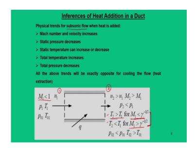
Now, something we talk about the subsonic flow. So, in the same logic when a subsonic flow which is at the inlet condition 1, condition 2 is mentioned here. So, for an inlet condition 1 when the flow is subsonic and it is entering to a constant area duct in which heat is added; so what will it make? In the downstream conditions, it would be such that the Mach number will increase, static pressure will decrease and this is most significant part for this subsonic flow about the temperature.
