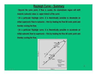
So, finally, we can summarize from Rayleigh curve that it is theoretically possible to decelerate a initial supersonic flow to subsonic flow; first by heating the flow till sonic point thereby, cooling the flow. In particular Rayleigh curve it is also theoretically possible to accelerate an initial subsonic flow to a supersonic flow first by heating till sonic point thereby, cooling the flow.
