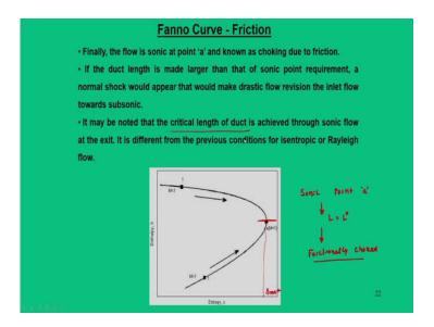
Now finally, when I reach the sonic point, the flow is choked. Sonic point a we say L becomes L\*, the flow is frictionally choked, which means physical inference that adding length or increasing the friction in a supersonic flow will lead you a sonic state.
