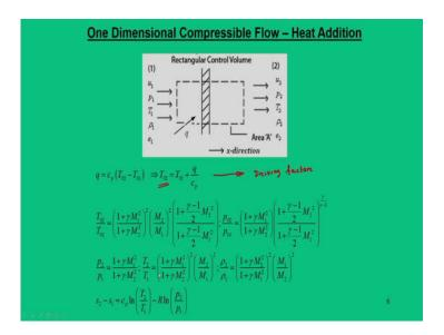
So, in the similar logic when you dealt with one dimensional flow with heat additions; that means, in a one dimensional duct when certain amount of heat is added, it changes the flow properties. So, this heat addition what it does in this case is; increases the total temperatures.
