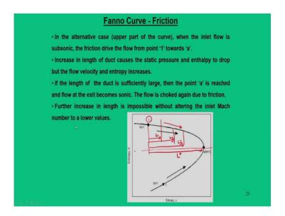
The alternative case when the flow is in the upper part of the curve. So, likewise in this upper part of the curve when I am at point a, the length addition will take me towards the sonic point. So, each point will give different  $L_1$ ,  $L_2$ ,  $L_3$  and finally, I will come back to this point as  $L^*$ .
