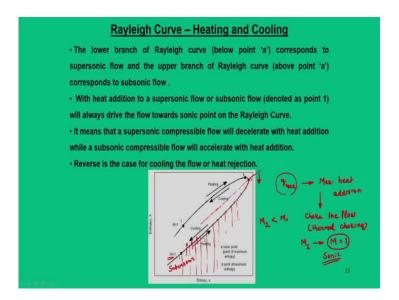
Now, let us talk about one by one; that means, we are in the lower branch of the curve. So, I am dividing this curve as two branch and I am in the lower branch of this curve. So, when I am lower branch of the curve that means obviously, we are in the supersonic region.
