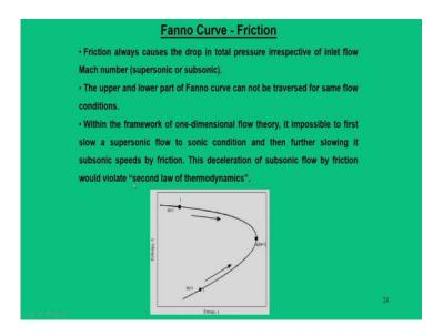
So, one can finally summarize that the friction always drives the flow towards sonic state with a drop in total pressure irrespective whether the flow is supersonic or subsonic at the inlet state. The upper part and the lower part of the Fanno curve cannot be traversed back for same flow conditions.
