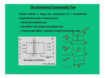
So, in the beginning of this one dimensional flow analysis, we introduced a constant area duct and we said there are three possible ways in which the flow properties from upstream and downstream conditions can be altered.
