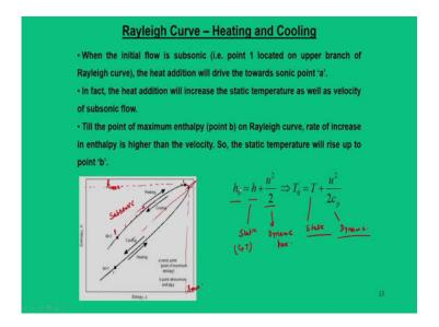
Now, let us see that what happens when heat addition process takes place for a subsonic flow. So, that means, when we are talking about the subsonic flow, we are now in the upper half of the curve. So, here we have subsonic. So, for an arbitrary states point 1 if I locate a point 1 here; so, heat addition will drive me to go in this path and cooling this flow will take me in the opposite path.
