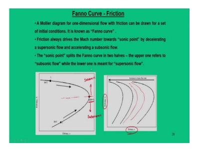
Let us see how we can give a thermodynamic definition to this. So, such definition is possible through a curve which is known as Fanno curve. So, the Fanno curve is nothing but Mollier diagram, which is drawn for a one dimensional flow with friction. And this particular curve shows here that in the similar way it is plotted in enthalpy entropy plane and for a given mass flux, there can be a Fanno curve. So, likewise different Fanno curves can be drawn for different mass flux rate.
