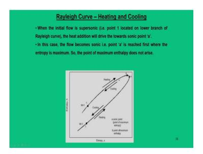
So, this point also I am already mentioned. When you are initial flow is supersonic the heat addition will drive the flow towards the sonic point and for this case there is no question of maximum enthalpy on its path, but it is not true when it is the initial condition is subsonic.
