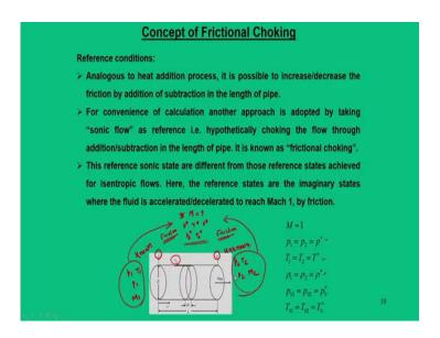
But the very basic point is that for a known conditions 1 and for a unknown condition 2; so, typically 1 is known condition, 2 is unknown condition means all flow parameters are known and all flow parameters of condition 2 are unknown.
