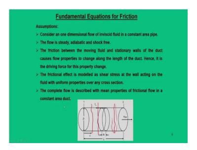
So, before you do with these fundamental equations, we try to say that there are certain assumption involved that is the flow is one dimensional in nature, but fluid is inviscid, but flow is compressible in a constant area pipe.
