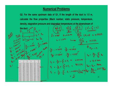
Now, moving further we are now in the next problem that for the same data, for the question 1; if the length of the duct is 1.5 metre, we have to calculate the flow properties.
