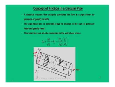
Now, just to give some brief introduction to the concept of friction in a circular pipe; we all know that the classical fluid mechanics problems involves a fully developed flow in a circular pipe. As shown in the figure, what do we have? We have inclined pipe. So, that there is a elevation difference between inlet and exit and this elevation difference is defined by  $\Delta z$ . So, if we say this is inlet and this is the exit.
