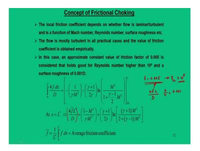
So, this is how we call this as a concept of frictional choking. Now, just to give some brief introduction about this frictional choking that the frictional choking is meant for the fact that flow needs to be sonic through addition or subtraction of length.
