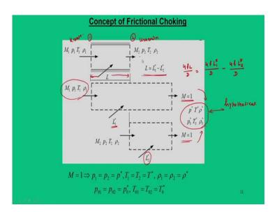
So, for that we can conceptually explain this particular fact in this manner that if we have a real situations 1 and 2 where the flow is entering in a duct or pipe of length L which is the actual length of the pipe and the condition 1 is known, the condition 2 is unknown.
