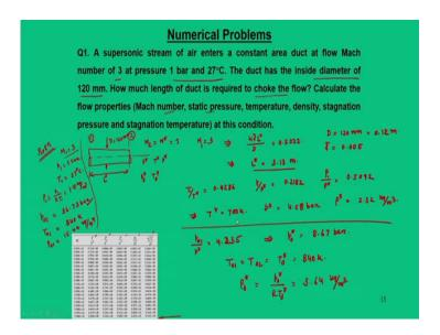
So, let us see that how this particular table can be used to solve some problems. So, a similar problem we have solved in a heat addition systems. We are now trying to solve the similar problem with respect to friction. So, there the parameter that was given is heat added to the flow. Here, the parameter that is given to us that addition of length.
