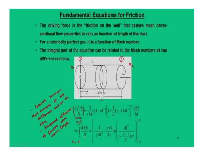
So, these equations after simplification, we are going to get a term in the form of Mach number. So, that means, in that previous equation the factor of interest is the term  $\frac{4f dx}{D}$ . This  $\frac{4f dx}{D}$  is now related to Mach number that is given by this expressions.
