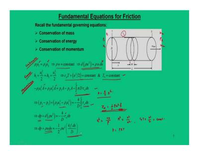
So, here we are going to revisit three fundamental equations; first is continuity. So, as you see that if you have  $\rho_1 u_1$  and  $\rho_2 u_2$ , the continuity equation holds good  $\rho_1 u_1 = \rho_2 u_2$  and since we are analysing in a differential section dx, so, I can express this term  $\rho u = \text{constant}$ ; from this expression you can evaluate a term what will happen to  $d(\rho u^2) = \rho u du$ . So, these things we are going to use in this subsequent analysis.
