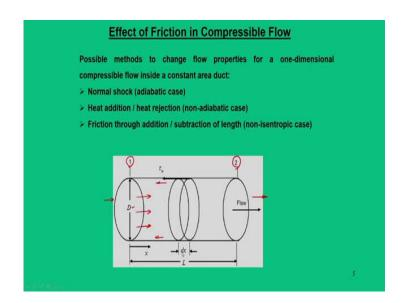
So, if you recall our previous analysis we developed some correlations for normal shock heat addition process and in fact, these two are the possible method to the change the flow characteristics in a one dimensional flow in a constant area duct.
