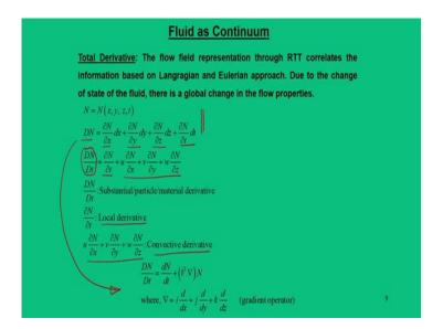
Now, the Reynolds theorem introduce a parameter which is called as  $\frac{DN}{Dt}$  and it happens to be a mathematical term which we called is as a Total Derivatives. So, to solve this mathematical term, we have a tool which is mathematically which is represent this DN in terms of dx, dy, dz and dt. So, this is a mathematical expression that comes for a given properties.
