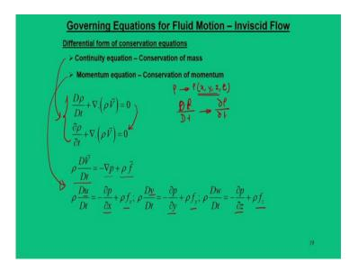
Now, we will talk about this the differential form of conservation of equations and that is continuity and momentum equations. In this slide, there are two equations given one is for continuity equations and the second one is the momentum equations.
