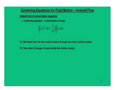
Now, when you deal with this, when you do this and apply this equation; then, the integral form of conservation equation that is conservation of mass as two terms; left hand side and right hand side. The left hand side term represents a surface integral which is the net mass flow rate into the control volume through the entire control surface. The second term or right hand side of this term is a volume integral which is the time rate of change of mass inside the control volume.
