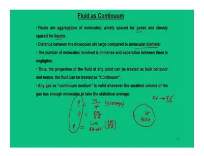
Now, going for the concept of fluid as continuum. So, when you say fluid as a continuum which means that the fluid has certain number of molecules which is occupied in certain volume and these number of molecules are sufficient enough to take the statistical average of any fluid properties.
