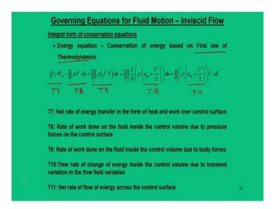
And the next part is the energy equations, which is based on the first law of thermodynamics. So, if you look at these expressions, here we are the term that is energy consisting of internal energy, kinetic energy plus potential energy. Here, we have not mentioned about the potential energy because we are not we will not be dealing with this.
