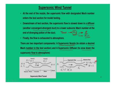
And, when the flow is exhausted to atmosphere it is close to the free stream pressure at the atmospheric conditions. And also, in the diffuser portion, there is another divergent section of the duct which is known as diffuser. And this diffuser has also a throat for which the area is  $A_{t2}$ , and here also it is nothing but the choked area or  $A^*$  and M is also attain 1.
