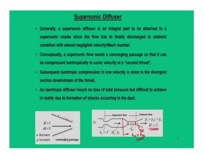
So in the reality what we are going to achieve is that we have to incorporate a diverging passage at the end of the test sections part. So if you see here, the test section parts ends at this point. So, when it is at this exit of this test section, the flow is already supersonic, so since the flow is already supersonic it has to enter a converging passage to slow down its velocity.
