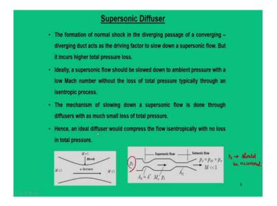
So, the formation of normal shock in a diverging passage of a converging diverging duct act as a driving factor to slow down the supersonic flow, but it incurs a higher total pressure loss.
