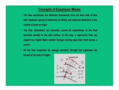
So, how is it done we can refer this particular figure; as we say that, in this particular example what has been seen shown here that a expansion corner is created. What does this mean? Means there are essentially there are two surfaces and these two surfaces are meeting at a point A. So, the supersonic flow passes through this surfaces which is horizontal that is the upstream of flow, region 1 and this flow has to turn through an angle  $\theta$  downwards.
