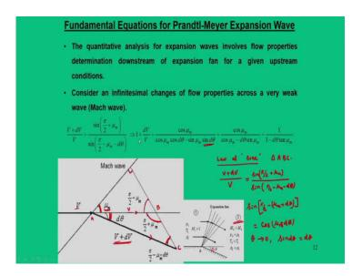
Now we will move to the fundamental equations for Prandtl - Meyer expansion waves. So, to start with the fundamental equation of Prandtl - Meyer expansion waves what we are going to see is that as I mentioned that the event of supersonic flow in an expansion process occurs through series of infinite Mach waves, we will take one such Mach waves.
