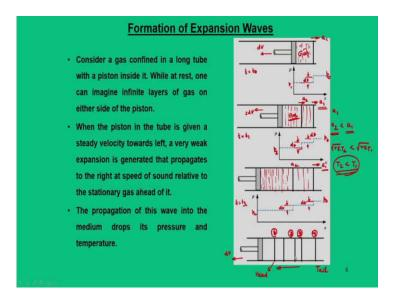
Now, to evaluate this particular concept of expansion process we will now discuss about the formation of expansion waves and likewise in previous cases what we do is that we take a piston cylinder device in which a gas is kept. So, in this case also we will say there is a gas which is kept in a piston cylinder medium.
