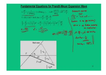
So, here this particular expression, we have to use some mathematical trick or expansion series, which means any equation  $\frac{1}{1-x}$ , where x less than 1 in an expansion series, we can write  $\frac{1}{1-x} = 1 + x + x^2 + \dots$  So, here replace x as  $d\theta \tan \mu_m$ . So, when I replace this so I can write  $1 + d\theta \tan \mu_m + \dots$  So, since  $d\theta$  is small. So, this means higher order series are neglected.
