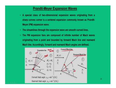
Now, having said this we will now define a special class of expansion wave known as Prandtl - Meyer expansion waves. So, these Prandtl - Meyer expansion waves are the a class of waves where we call this as a expansion fan and here the head and tail of the wave are defined through a Mach line. Or in other words we can say these are the waves that generated from a center point and there are infinite waves and all these infinite waves are known as Mach waves.
