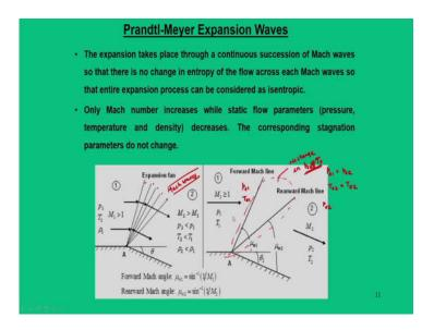
And since this is how I have explained all these things, the expansion waves takes place through continuous succession of Mach waves. So, there is no change in the entropy of the flow across each Mach waves and we say all these are Mach waves.
