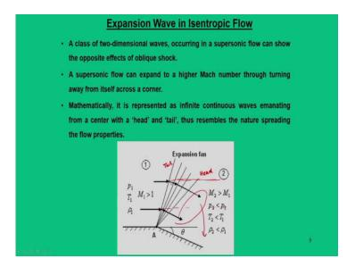
Since we say that the flow turns smoothly across an expansion wave. So, we can say that medium can be treated to be an isotropic medium.
