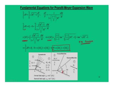
So, putting  $\frac{dV}{V}$  as a function of  $\frac{dM}{M}$ , then we can replace that equation and now we can integrate that equations from  $\theta_1$  to  $\theta_2$ . So,  $\theta_1$  to  $\theta_2$  in our case is nothing but our initial angle is 0. So, many a times  $\theta_1$  is equal to you can say it is 0. So, you can go up to  $\theta_2$ . So, we get a integral of this equations.
