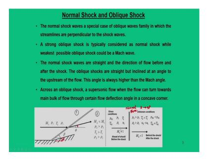
Now, when a oblique shock is formed? The first question arises that, when a supersonic flow encounters a compression corner and this particular compression corner what you can see in this figure is a type of concave corner which is inclined by an angle  $\theta$ . So, I can say that this corner is oriented by an angle  $\theta$ . So, when a supersonic flow sees this compression corner an oblique shock wave is formed.
