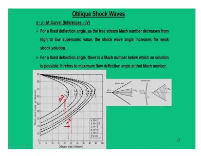
The next important inference that we can say is that, for a fixed deflection angle as the free stream Mach number decreases from high to low supersonic value. So, for a given deflection angle  $\theta$  let us say 20°; if I am moving from high supersonic, that is if I am moving from M is equal to 8 to M is equal to 2, what we see in the weak shock region, your shock wave angle increases. So, in the weak shock region, the shock wave angle increases.
