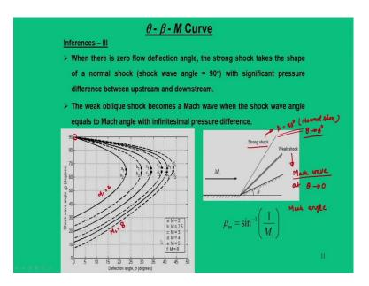
So this is how we say that what will happen when we are in this domain. But, let us see that for a given Mach number, what are the upper limits and lower limits? So, first upper limit I can say, when we say it is a strong shock; the strong shock becomes a normal shock when  $\beta$  is equal to 90°, we say it is a normal shock.
