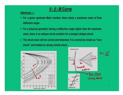
So, what it means to us? So, again we refer the same curve, so I will say that, the first inference that we are going to say is that; we are going across different Mach numbers ranging from 2 to 8, for a given upstream Mach number there is a maximum flow deflection angle that is  $a_1$ ,  $b_1$ ,  $c_1$ ,  $d_1$ ,  $e_1$  and  $f_1$ .
