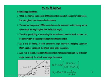
So, in other words what I have shown here is that from this  $\theta$ - $\beta$ -M curve, we can say using this relation, what parameters that controls? Whether a oblique shock will be a Mach wave or oblique shock will have a strong shock solution or oblique shock will have a weak shock solution that is mostly decided the parameter which is normal component of the Mach number.
