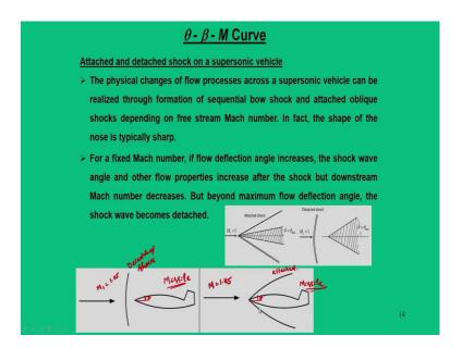
So, this is the another example what I am trying to give that, whatever I have summarized that in most of this supersonic objects or you can say missile of this particular shape; so you can say it is a missile, missile shape object. Now, when this missile shape object travels at a high altitude, at different altitudes it moves in different flow regimes.
