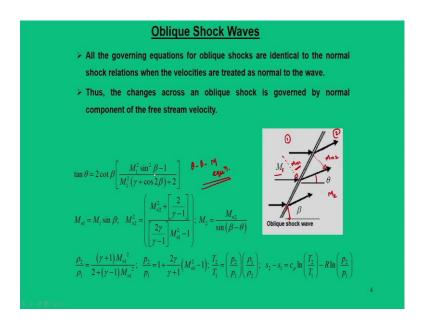
So, now with this oblique shock situations; like if your shock wave is angle is  $\beta$ , the flow deflection angle is  $\theta$  and upstream Mach number is M<sub>1</sub>; then, we derived in the last lecture some the fundamental equations and the summary of those fundamental equations are given here. So, what we have shown here is that, across an oblique shock, it is the normal component of the Mach number that becomes vital for flow property calculations.
