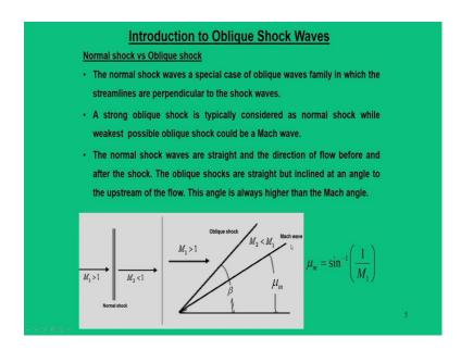
Now, just to give a brief a distinction between a normal shock and oblique shocks; what I can say is that, normal shock waves are special case of oblique shocks family in which stream lines are perpendicular to the shock waves. In general, the shock wave initiation start with a Mach wave which is a two dimensional phenomena. And one particular situation, the shock wave is normal to the flow; that means the direction of the stream line and the shock waves, they are perpendicular to each other.
