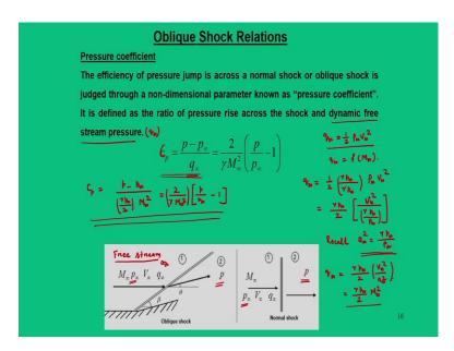
The next important topic is a term which we call as a pressure coefficients. So, as I mentioned in my previous lecture that a normal shock is treated as a compression device; because the static pressure always rises. And in fact across an oblique shock, the static pressure also rises.
