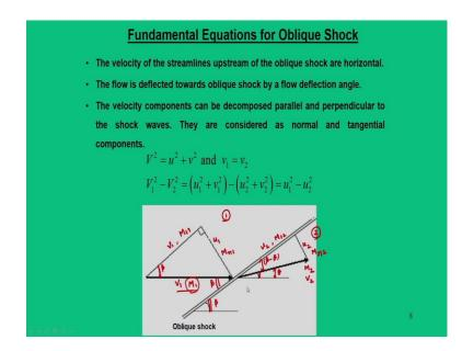
Now, we are going to analyze the fundamental equations for an oblique shock. So, to study this fundamental equations of oblique shock what we can say, we have to consider an oblique shock; this oblique shock is sitting at an angle  $\beta$  with respect to horizontal. And this is one particular streamlines which has a Mach number M<sub>1</sub>, velocity V<sub>1</sub> and it after it crosses the oblique shock, the flow turns; that means stream line turns to an angle  $\theta$ .
