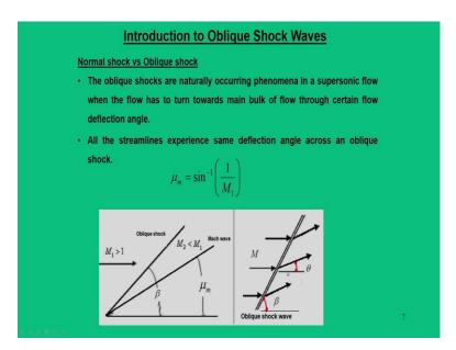
The most important phenomena of an oblique shock is that, this is a mechanism across which the flow can turn. So, what happens in a normal shock, flow does not turn; because this streamlines before the shock and after the shock they are perpendicular to each other, so they do not turn.
