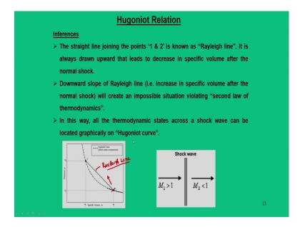
So, now when I join this line 1 and 2 in this Hugoniot curve. So, this line is known as Rayleigh line. Because, it is drawn for a particular mass flux. And, in fact, I told that the downward slope of the Rayleigh line is not possible, because we cannot go below this line.
