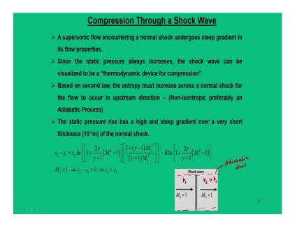
To do this analysis let us see that when we undertake a compression in a shock waves. So, we say there is a standing normal shock. So, across a shock wave the Mach number drops, but your static pressure  $p_2$  always rises, but in a very steep manner. Now, one angle we can give to this particular problem and obviously this process cannot be considered as any of the quasi static process, because this jump is very instantaneous or very steep. And, this happens in a very shortest time.
