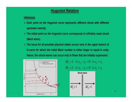
So, to start this, one can say that one can draw an Hugoniot curve of like this in a pressure specific volume diagram. So, for different values of  $p_1, \vartheta_1$  one can find out all possible numbers. Now, when I say so, next question arises, where is this initial point?
