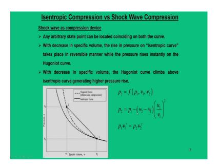
So, this is how I have explained so far that how a shockwave as a compression device can be interpreted? I mentioned that with decrease in the specific volume rise in pressure in isentropic curve takes place in a reversible manner where pressure rises instantly on a Hugoniot curve. With decrease in the specific volume the Hugoniot curve climbs above the isentropic curve; that means, it generate a high pressure.
