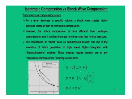
So, one can make summary of this analysis that why a shock wave compression is a effective method. So, one of the key point is that for a given decrease in this specific volume, that is  $\vartheta_2 - \vartheta_1$ , the shock wave creates higher pressure rise increase than the isentropic compression.
