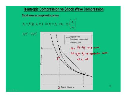
So, to do that one interesting thing what we can say that we can bring a concept as shock wave as a compression device. So, what I did is in the same Hugoniot curve, I superimpose this isentropic curve; that means, when I am starting from same point 1 and I try to go on a Hugoniot curve that is dotted line, and from same point I also can start my compression journey in the isentropic curve.
