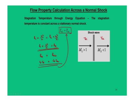
Another important relation that we are going to talk about the stagnation temperatures. So, we say the before the shock it is  $T_{01}$ , after the shock it is  $T_{02}$ . So, as I say that energy equation does not change; so I can write  $h_1 + \frac{u_1^2}{2} = h_2 + \frac{u_2^2}{2}$  and we also know  $h + \frac{u^2}{2} = h_0$ .
