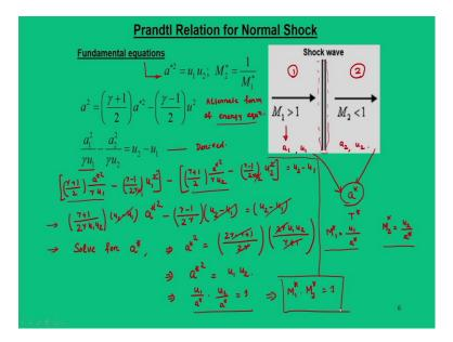
So, this particular equation we derived and we also want to use the another form of equation, that is alternate form of energy equation. So, if you recall this alternate form of equation where did you get? In our isentropic flow situations, we derived the equation in which we involved the speed of sound, the velocity of the flow and star conditions in one form of these equations.
