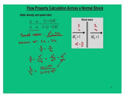
The next expression that we are going to talk about is the static density and speed ratio. So, now we are moving with the fact that, we are going to calculate the flow property across a normal shock. So, for this flow property calculations the very basic relations that you have to remember is the Prandtl relation. So, these Prandtl relations will say that  $a^{*2} = u_1u_2$ . So, this relation will be very vital for these calculations.
