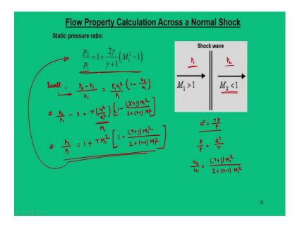
Now, we will move to the conditions for static pressures. So, very basic things that we want to say the static pressures are defined as  $p_1$  and  $p_2$ , that is before the shock and after the shock. So, our basic philosophies that we want to find out the ratio of  $\frac{p_2}{p}$ . So, this
