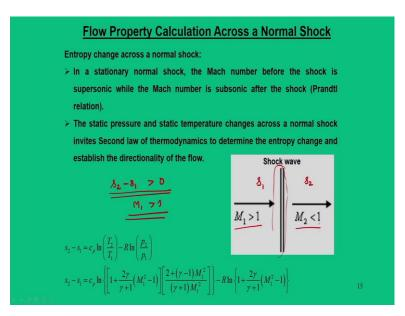
Then we are going to move a very important calculations that is entropy in the flow field. So, as you know that across the shock wave, the entire flow field is non isentropic. So, if I say absolute entropy before the shock is  $s_1$ , if I say absolute entropy after the shock is  $s_2$ that is per unit mass. So, we can easily calculate what is happening
