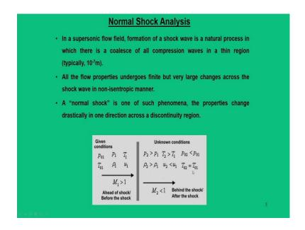
Now, just to brief about what we have framed the concept of normal shock. What we can say is that; normal shock is a inevitable phenomena in a supersonic flow field and, it occurs naturally by the merger of all compression waves in a very thin region. And, this thin region is typically measured to be a size of 10<sup>-7</sup>m.
