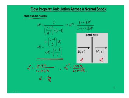
So, in the previous relations the Prandtl number talks about the relation between  $M_1^*$  and  $M_2^*$ . But, it does not talk about what is relation between M<sub>1</sub> and M<sub>2</sub>. But, we know that any arbitrary Mach number can be correspondingly connected to its star condition of Mach number, that is through this expressions.
