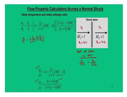
Now, then next point we are going to address is the static temperature and enthalpy. So, here if I define this static temperature as T<sub>1</sub> and T<sub>2</sub> that is one is before the shock, other is after the shock and static enthalpy  $h_1 = c_p T_1$  and static enthalpy  $h_2$ , after the shock will be  $c_p T_2$ . Also we have to write equation of state, that is we can write  $p = \rho RT$ .
