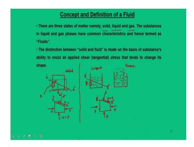
The next part is the first part or what we say is the concept and definition of fluids, but before you go for those definition of fluids, it is the most important concept of matter that exist in three different states, so that is namely solid, liquid and gas. So, the substances that are in liquid and gas phase they have a common characteristics and they are called as fluids.
