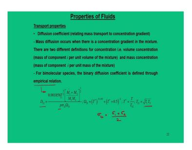
But, however, one particular interest we want to say that when you deal with the high speed flow of gases of then when a one gas tries to diffuse into other, then we would call this as a coefficient called as a binary diffusion coefficients which is calculated by this expressions  $D_{12}$  and, it is empirical relations.
