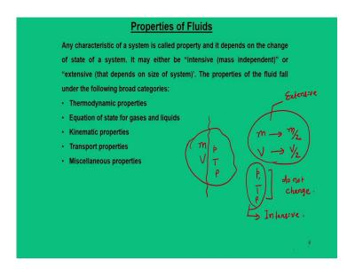
Now, moving back to the this the next part of this lecture, which is properties of the fluids. So, the thermodynamic definition of the property of a fluid means it is a characteristics of the systems that depends on the state of a system. So, these properties may be intensive which is mass independent or extensive with that depends on the size of the system.
