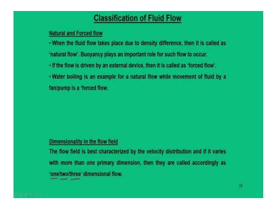
The other type of flows are of interest many times is a natural flow. Natural flow and force flow; natural flow is normally buoyancy driven for example, water boiling is a kind of a natural flow and when the fluid is driven by some external agency that means, whenever there is a pressure difference mechanism which is being put so that the flow can occur. So, such a flow we call this as a force flow.
