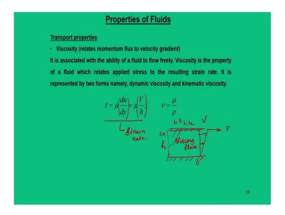
So, the first properties is the viscosity, it relates the momentum flux to the velocity gradients. So, essentially the viscosity is the term which is defined as the ability of a fluid to fluid flow to flow freely.
