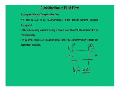
Here our main focus comes into it which is incompressible and compressible flow. So, essentially in our entire domain we will be mainly looking at the flow nature which is the compressible. So, under what circumstances we say the flow to be compressible whenever there is a flow occurring in a system or in a duct system and are two arbitrary locations.
