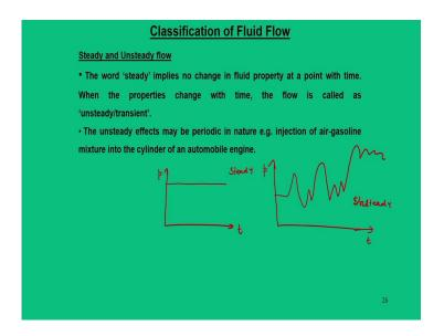
Other type of flows that is steady flow and unsteady flow: so, when you say steady flow when you say steady flow we essentially see how the parameter is any fluid parameter which is changing with time. So, let us say pressure we are, but let us say I am plotting pressure with respect to time, at any in a space medium so, I will see that the pressure do not change. So, it is a steady.
