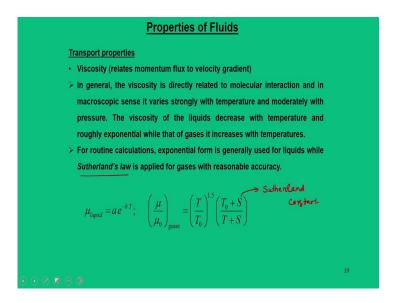
The other properties of importance which is the now when we actually calculate the viscosity for the gases, it is seen that the for gases the viscosity increases with the temperatures. So, many a times when we deal with very high temperature flow gasses, we need to find out how viscosity changes with the temperatures.
