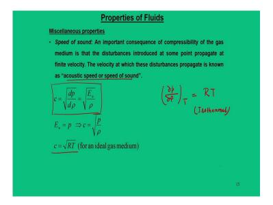
The next important properties which is called as speed of sound, this parameter we will be looking at in more exhaustive form in the subsequent class. Just for the sake of continuity I am just explaining that the one of the important consequence of compressibility of gas is the fact that when a gas moves in a medium it creates a pressure disturbance and these pressure disturbance moves at certain speed which is known as the speed of sound or typically known as acoustic speed.
