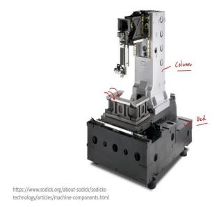
Now, let us see where these casted components are used in the automated system. In the slide, we can see the interior of a CNC machine tool. There are various structural elements that we can locate such as the bed of the system, the column. There are more elements which are mounted on the bed over which the table will be mounted. All these elements cannot be outsourced. We have to design them and we have to fabricate them in house.
