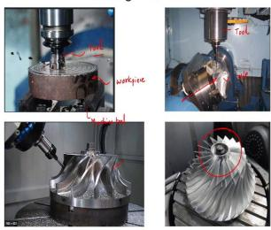
Milling is the most versatile manufacturing operation. In the milling process a rigid tool is used. The strength of the tool is much higher than the workpiece. There is a relative motion between the tool and the workpiece, and the mechanism or machinery which is providing the relative motion between the tool and the work piece is called as the machine tool.
