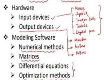
CAD can be defined as the integration of computer science techniques for the engineering design. The CAD systems require certain hardware and specialized software. What are the hardware elements required to have the CAD system? The input devices and the output devices are required. The input devices are a typical mouse or joystick, tracker balls, tablets, digi pens or digital pens.
