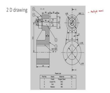
Let us look at what are the modes to visualize the product in the digital environment. The first mode of visualization is in a 2 dimensional mode, on our screen we can see a crank assembly. this crank assembly is being shown by using 2 different views. For 2D modeling, multiple views are needed, more than 1 view is required to communicate the information about the product.
