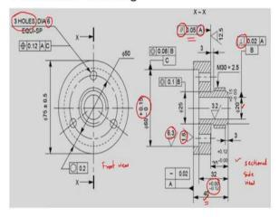
On the screen wecan see a typical production drawing which has 2 views. We can see a sectional side view and the front view. This is the front view of the wheel and this is the sectional side view. In addition to the dimensions, the tolerance values are also provided.
