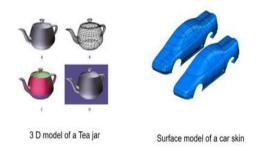
On the screen we can see the variety of ways to visualize the object. This is the wireframe model and this is the surface model or the solid model. We can attach colors to the scheme of the solid model and even we can attach the materials. In 3D modeling we can render the objects we can have the effects of lighting. A typical surface model of a car skin is shown on the screen.
