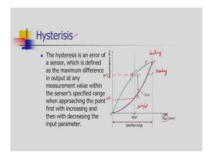
The next performance related term is hysteresis. The hysteresis is an error of a sensor which is defined as the maximum difference in output at any measured value within the sensors specified range when approaching the point first with increasing and then, with the decreasing the input parameter. We are using certain sensor for increasing trend of the field variable to measure the response when the field variable is having increasing trend.
