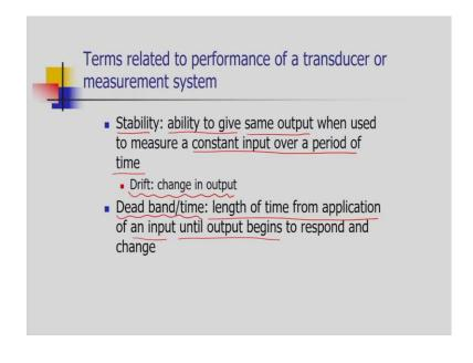
Stability is defined as the ability to give the same output when used to measure a constant input over a period of time. Let us consider an example of a furnace where the continuous heating is carried out at a constant voltage induction furnace.
