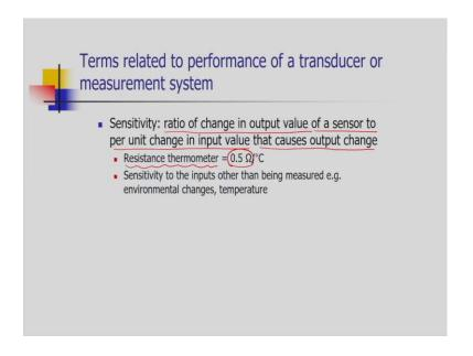
The next performance related term of a transducer is the sensitivity. It is defined as the ratio of change in output value of a sensor to per unit change in input value that causes output change. Considering the example of a resistance thermometer, if there is a change in 1 °C in the environment, then the instrument is reading or the instrument is giving an output of 0.5 ohm. That is called as the sensitivity.
