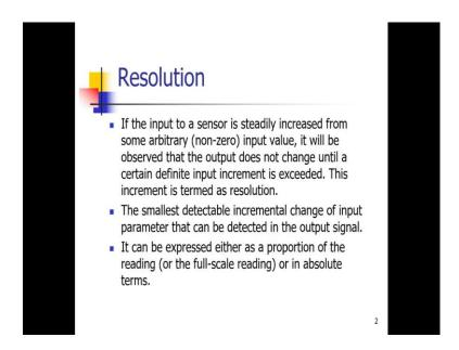
The next term associated with the performance of a sensor is the resolution. It is defined as if the input to a sensor is steadily increased from some arbitrary input value, it will be observed that the output does not change until a definite input increment is exceeded. This increment is called as the resolution.
