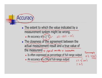
The next term of the performance of a sensor is the accuracy, which is widely used. The accuracy of a sensor can be defined as the extent to which the value may go wrong than the expected value. If it is said that the accuracy is  $\pm$  2 °C in a thermocouple, it means that if a thermocouple is giving me a temperature of say 25 °C; this 25 °C is having an accuracy of  $\pm$  2 °C.
