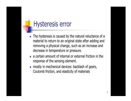
Now, let us see why this hysteresis error is generated. The cause of the hysteresis error is due to the natural reluctance of a material to return to an original state after adding or removing a physical change.
