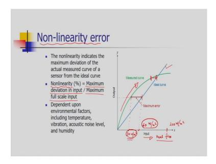
What are the reasons due to which we are getting the non-linearity error? These non-linearity errors are due to the environmental factors such as temperature, vibration, acoustic noise level and the humidity.
