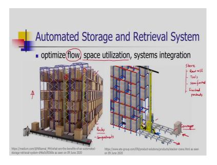
Now, as far as automation in manufacturing is concerned, the next type of equipment which is very common and important is the automated storage and retrieval system, which consist of a rack and a stacker crane.
