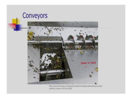
In this case screws are used. Stainless steel screws are used. Stainless steel is a good quality food processing material and here we can see the grapes which are to be conveyed and further crushed to produce the wine. The grapes that are to be moved are shown in a stainless steel screw conveyor.
