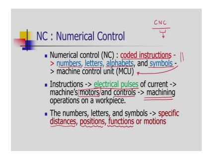
To machine these complex surfaces, we need Computer Numerical Control technology. The CNC technology or the term CNC has 3 letters C and N C. What is the meaning of N C? N C is Numerical Control. In this numerical control, coded instructions are used. These coded instructions have various numbers, letters, alphabets and symbols.
