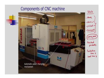
The next type of arrangement that is required in CNC machine tool is the pallets. Pallets are used to stack, store, protect and transport the work part. We need to stack the work parts, stack the finished products, store the work parts and the stored work parts will be fed to the machine whenever and wherever it is required. On the pallet, various work parts are mounted and the machine will carry out the processing operation like machining or drilling or welding.
