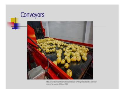
The next type is the belt type of conveyor with sufficient frictional coefficient to carry or to convey the food products. The belts should be of food grade quality which should not contaminate the food products. Potatoes which are to be moved on the belt conveyor are shown, which may be utilized for its processing further.
