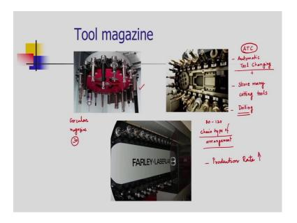
I In a typical conventional machine tool; very limited number of cutting tools can be mounted, which have to be changed manually. This is a time consuming task. In CNC machine tool operations, we use Automatic Tool Changing facility or ATCs. In addition to that we should hold multiple number of cutting tool.
