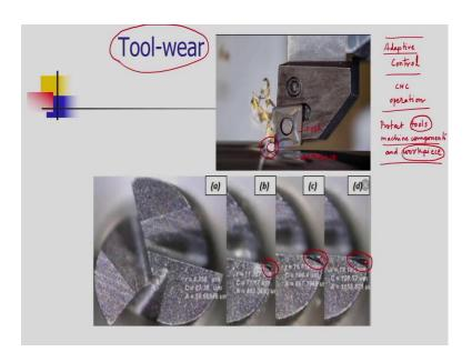
Some of the advanced concepts are coming in the CNC machine tools. These are adaptive controland its usage in the CNC operation. What is the meaning of the adaptive control? In adaptive control, the tool, machine, work piece are protected from the damages caused by the malfunctioning of the machine.
