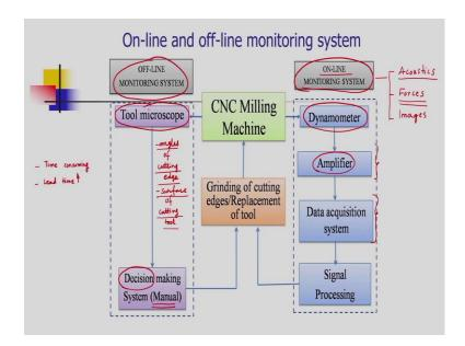
What are the ways or what are the methods to monitor the cutting tool failures or to monitor the cutting tool health? Basically there are two methods; first is the offline monitoring system. In offline monitoring system, the cutting tools are taken out from the spindle and then these cutting tools are observed under the tool microscope.
