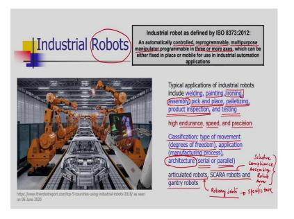
A very important automation equipment is the industrial robot. A industrial robot as far as ISO 8373:2012, is defined as an automatically controlled, reprogrammable, multipurpose manipulator. It is a mechanical equipment controlled by electronics. It is a
