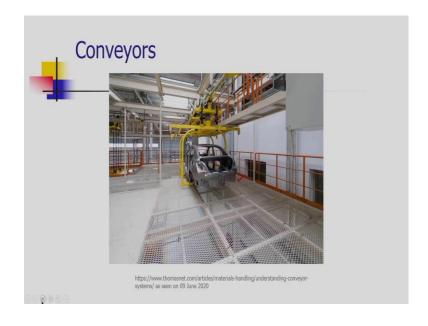
A overhead conveyor is shown and this overhead conveyor is used to convey the car body. The car body is mounted on a carrier which moves by a mono rail mounted on the shop floor. In this way we can save the floor space and have the easy movement of the heavy bodies which are hanging inside the shop floor. Thus, the floor space can be utilized for other operations.
