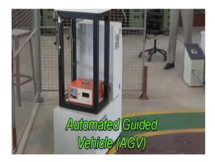
The figure shows an automated guided vehicle. This automated guided vehicle is moves and reaches to its destination, the components are then taken through the conveyor on automated feeding system.
