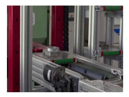
All the racks are coded. Here we can see the racks are C 1 R 3. C 1 means column 1 and R 3 is row 3. Thus, column 1 row 3 is the rack number.
