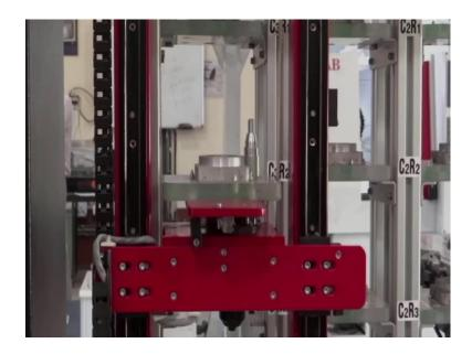
Now, this stacker goes inside, it takes the components that to be machined in the flexible manufacturing system. The components are then taken and these components will be fed to the conveyor, which will take the components and load the automated guided vehicle.
