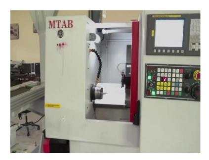
The turning operation means, there is reduction in the size, reduction in the diameter of the axisymmetric parts.
