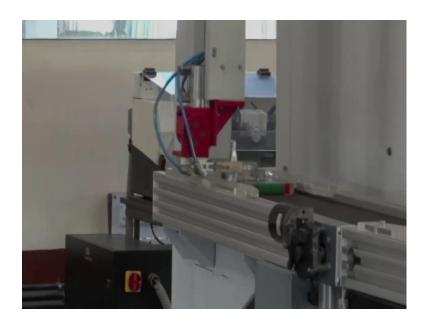
The first operation will be carried out on the CNC turning center. The automatic feeding system has taken the component that is to be turned on the CNC turning center.
