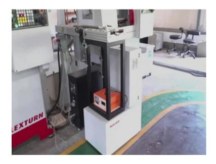
The conveyor then moves and comes to the pallet, it will get loaded on the top portion of the AGV. Now, the next work part will be processed on the CNC milling center. Again, an especially designed feeding mechanism will approach the work part.
