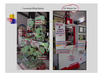
However, the conventional milling machine is having a drawback that very high level of surface finish, freeform surfaces cannot be manufactured, and it is very difficult to achieve the accuracy or the resolution in microns. The reason is obvious that there is human intervention and it is difficult for a human being to control the feed that is to be given to the work piece.
