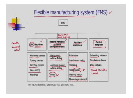
Let us move ahead and look at what are various elements or what are various types of equipment which are the part of the FMS system. The first group of equipment or the first group of machines is the CNC machine. CNC is nothing but Computer Numerical Control machines.
