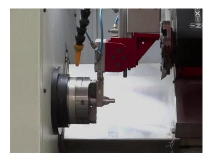
The component has been taken and will be feed to the machine. The machine has a three jaw automatic chuck (chuck is holding the component). It is a pneumatic operated chuck, the feeder will leave the jaw and immediately the chuck will hold the jaw. The component is now held in the chuck.
