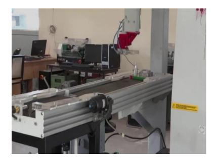
The feeding mechanism will orient the work part in its original position and then it will be put on the conveyor system. The conveyor system will load the finished or the semi processed work part to the AGV.
