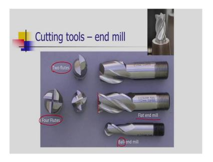
Milling tools may have two flutes or two cutting edges or it may have four flutes or four cutting edges. There are many tools which have a flat end and are called as flat end mill. When the tool end is of ball shape, it is called as ball end mill. Variety of such tools are used to generate various complicated surface using the milling operation.
