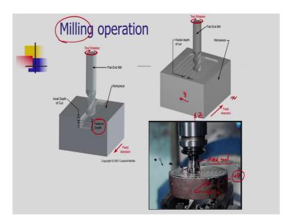
In order to understand the CNC machining center, we have taken here the example of CNC milling operation. Milling operation is a material removal operation, in which a
