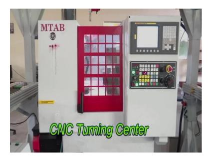
The machine door will be automatically closed. The central computer will now give the instruction to the CNC machine tool to carry out the desired manufacturing operation.
