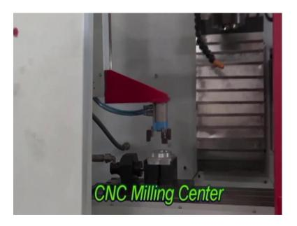
The GMN code will get executed and then the process part or the machine part will be ready for its further operation. The same feeding mechanism is approaching the work part. It takes the work part and that work part will be put on the conveyor for its further transfer to the automated guided vehicle.
