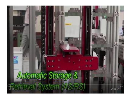
Afterwards we will be shown, one by one what are the various equipment used. In the figure, an automated storage and retrieval system and a crane stacker can be observed. The retrieval system is having a crane stacker.
