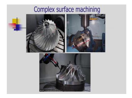
A turbine blade is shown as an example. The shape of the turbine blade is complicated. All the blades are thin, they are intact with its core and are precise as per as their thickness is concerned. Their shape is so complex that it is very difficult or rather impossible by using the conventional machine tool to carry out this operation. Hence, for this purpose, multi axis CNC machine tools like the five axis CNC machine tools are used. .
