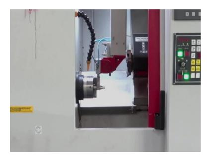
After machining of the work parts or after processing of the work parts, the same feeding mechanism will approach the work part, the chuck will open and immediately the feeder will hold the work part and will safely unload the work part from the CNC turning center.
