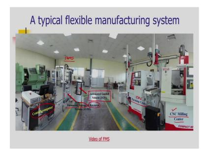
Now, let us see how a typical flexible manufacturing system works. For that purpose, on the figure, a typical arrangement is shown, where the various elements of the flexible manufacturing systems are shown. These are CNC machines. Here in the figure, a CNC milling center, a turning center can be observed.
