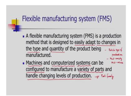
Beginning with the definition of a flexible manufacturing system, there are three types of productions being used in the industry; low production, medium production, and high volume production. In medium production, there is a variety of components need to be manufactured and the volume of the production is in medium range.
