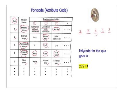
Let us find out how to define a polycode of a typical product. To understand the concept, let us take the example of the same spur gear that we have seen for the monocode.
