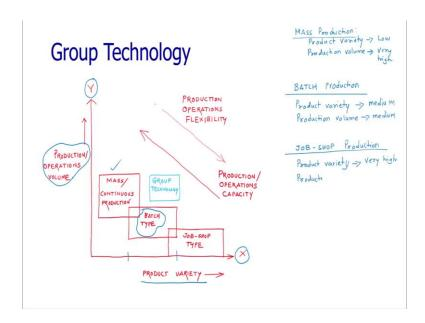
If we start looking at the variety of type of productions which are carrying out in an industry or in an enterprise, we can divide this type of productions into basically three categories or three groups. To understand this, let us take the product variety along the X axis and production operations volume along the Y axis.
