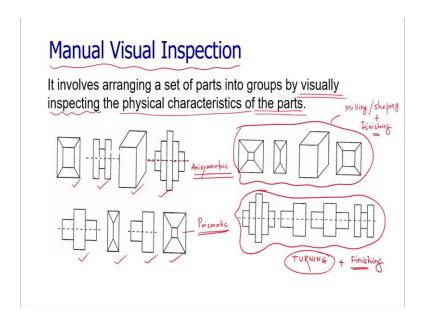
Looking at the first method that is Manual Visual Inspection method. Basically, the manual visual inspection method as I mentioned, we are making a groups, we are making sets by visually inspecting the physical characteristics of the part. Here we are making the visual inspection and the physical attributes of variety of parts. To understand the process, let us look at a number of products which are in front of you.
