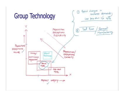
The first case is rapid changes in customer demands. It leads to low product life cycle. When the product life cycle is low, we cannot manufacture the products in bulk and just store in the warehouse because we do not know whether there would be consumption of the entire products that we manufacture. We have to take the decision based upon the demand in the market.
