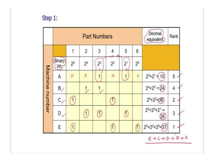
For that purpose as the rank order clustering algorithm is saying that we have to assign the binary weights; binary weights for the rows. To assign the binary weights for the rows, we have added one more row here and that is the binary weight row.
