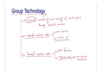
Now, how these group technology principles can be applied in the manufacturing; how we are applying the GT in the manufacturing? We got a cluster of products, we got cluster of machines and now how to move ahead. For that purpose, there are basically three modes or three prominent application. The first application is informal scheduling and routing of similar parts through selected machine.
