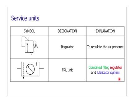
The entire FRL unit, the service unit, which is having the filtration, regulation and lubrication facility is together can be shown by using a symbol, which is there on your screen all the three functions operations are combined together. This is to enhance the convenience of using this facility.
