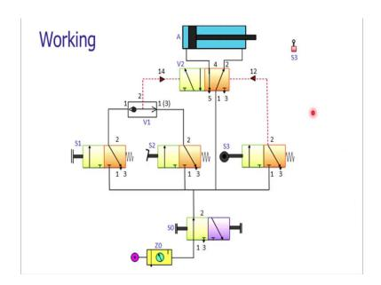
As it is mentioned that for displacement of the work parts or the components, which are there in the magazine, we need to have a double acting cylinder. A is the double acting cylinder which is to be controlled or which is to be operated by using the compressed air. We need the the compressed air which is being taken by the receiver tank and there is the FRL unit. From the FRL unit, the compressed air is taken.
