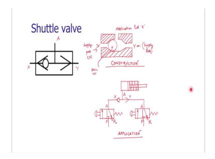
When we want to have the actuation of the actuators say, a single acting cylinder or double acting cylinder by using two different valves, then a shuttle valve is used. The shuttle valve is having three ports the port X, port Y, and there is the application port A. At port X the supply from one valve has been given and the port Y, there is another supply will be given by the other valve.
