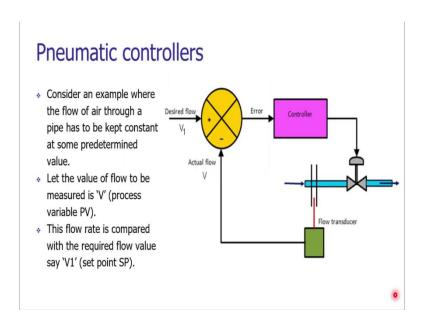
Now, to control the flow of the pneumatic energy or the compressed air inside a mechanical system, we are using the controllers. Let us consider an example where we need to control the flow of air through a pipe. We need to have a constant supply of the compressed air at the application. To have the controlling of the constant air or to apply the constant air, we are using a controller, but this controller is working upon the input which is the error.
