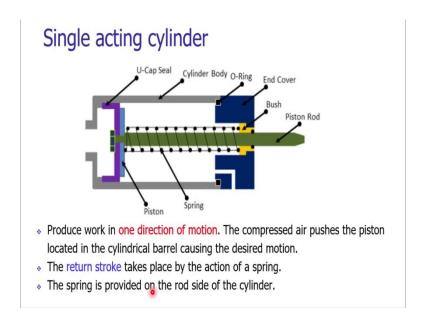
A typical single acting cylinder can be seen on your screen. It is single acting means it is producing the work in only one direction. The construction can be seen on your screen, it is having the cylindrical body. Inside the cylindrical body, there is the piston rod and at the end of the piston rod, there is a piston attached.
