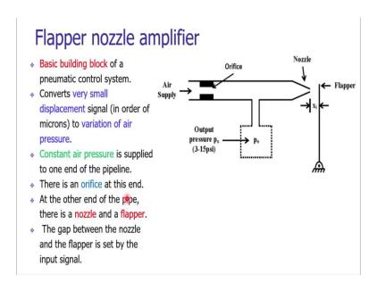
The flapper nozzle arrangement is the basic building block of the pneumatic controller system. It is basically converting a very small displacement signal into the variation of air pressure. The arrangement of flapper nozzle amplifier can be seen on your screen. We are having a tube and this tube is getting a supply of the pressurized fluid compressed air.
