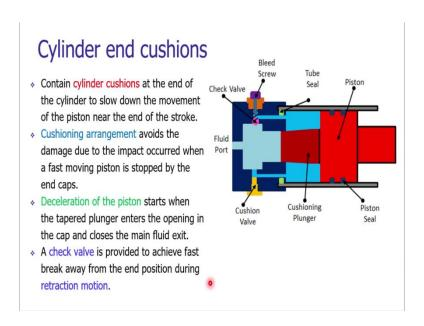
When the pistons are moving in a very rapid way, there may be chances of having the ramping of the piston at the walls and at the end of the cylinder, which are having various walls. Thus, to protect the ramping or the sudden impact of the piston at the end of the cylinder arrangement, cylinder cushions are used.
