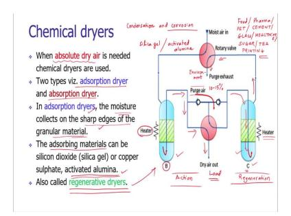
The next type of drying is based upon using the chemicals, variety of chemicals are used. Basically, the drying operation is used for the condensation and to avoid the corrosion. As we know that the moist air or the moist air which is having the water particles, water particles are promoting the chemical reaction and physical erosion. We need to remove the water particles to pass through the pneumatic systems.
