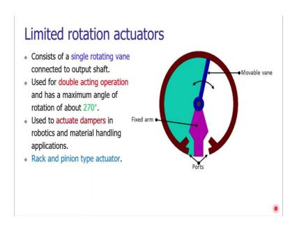
The compressed airs are also providing us the rotary motion and the devices which are converting the pneumatic energy into the rotational motion are called as the rotary actuators or rotation actuators. A typical arrangement of a rotation actuator can be seen on your screen.
