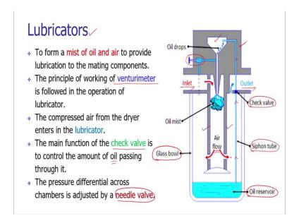
The next type of treatment of the air is lubrication, the lubricators. The dried air is stored in the tank and further it will be utilized for the desired application. During the passage, many mechanical elements need to be lubricated. For that purpose, we are deliberately adding the lubrication oil and creating a oil mist which is utilized for the mechanical operations of the valves or the actuators of the pneumatic system.
