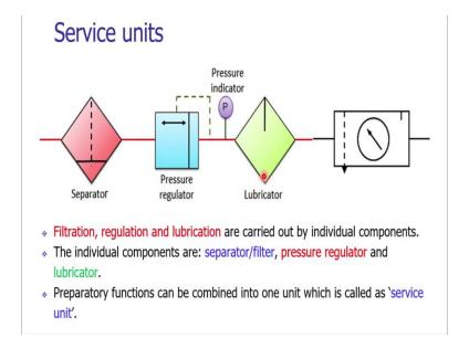
As we have seen that we need a separator, a pressure regulator and lubricator. These are the essential elements of the treatment of compressed air. In general, in the industry, the separator, pressure regulator or the lubricator, separator is also called as the filter so, filter, regulator and the lubricator that is called the FRL unit.
