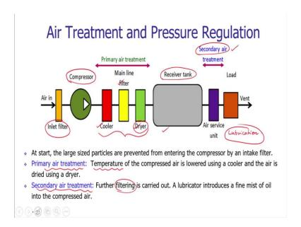
In our previous lecture, we have seen various types of compressors which are used to generate the pressurized air or the gas. After getting that compressed air, we are storing the compressed air in a storage device that is a tank and when we store the compressed air in the tank, we are processing, we are treating that air.
