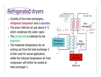
We can have variety of the air dryers. Mostly, the refrigerated dryer is used which is based upon the heat exchanger principle. We need to dry the air and that dry cool air will be utilized for the applications. In the refrigerated dryers, the cold air is used to reduce the temperature of the moist air so that the water particles will get condensed.
