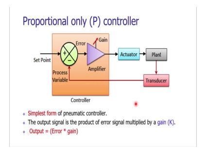
A typical proportional only controller schematic is there on the screen. Basically, we are trying to learn how to control, how to have the controlled application of compressed air at the desired level.
