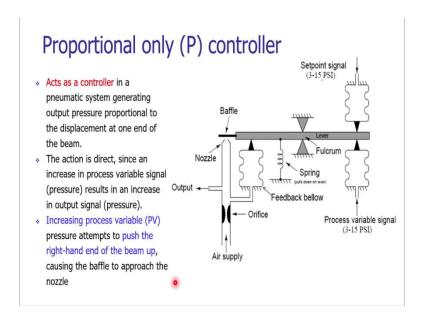
The typical proportional only controller based upon the pneumatic applications can be seen on your screen. Basically these type of controllers are used to generate the output pressure in proportional to the displacement of one of the end of the beam. Now, here we can see there is a lever, or a beam and that beam is fulcrumed.
