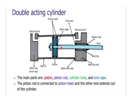
The double acting cylinder is providing us two; two-way action the forward stroke and the reverse stroke and both the strokes are being controlled by the compressed air only. The construction of the double acting cylinder is little more complex, but the elements are the typical elements.
