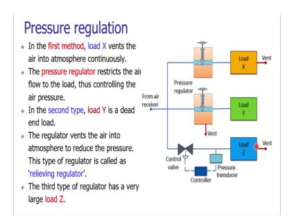
The compressed air is having variety of application in the industry. In certain cases, we need to have the continuous passage of the compressed air. Let us consider the ventilation purpose. During such kind of application, from the load itself, the compressed air is getting vented out. For such application, we are utilizing a simple pressure regulator which is regulating the pressure of the compressed air at the load.
