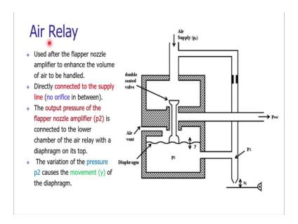
Air relay is one of the building blocks of the pneumatic based controller and it is using the flapper nozzle amplifier to enhance the volume air handling methodology to enhance the volume of air to be handled during the relaying operation.
