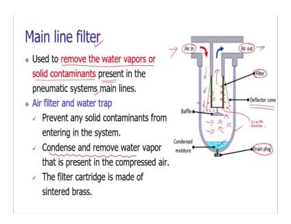
One typical filter is the main line filter and it just removes the water vapor or solid contaminants which are present in the pneumatic system main lines. The construction can be seen.
