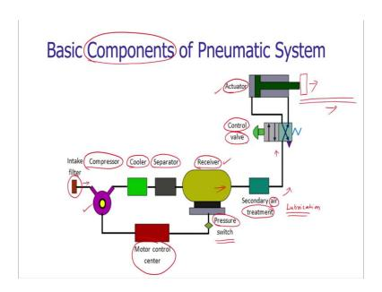
Let us see what are the various basic components pneumatic system has. The fundamental components of the pneumatic system is the compressor which takes the air from the environment and then it increase its pressure, it reduces its volume and it increases the temperature. When it takes the air inside for the increase in its pressure, it needs to filter.
