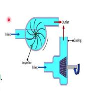
The next category of the compressor is the dynamic compressor. They are non positive type, where we are getting large volume of compressed air which is in general required for the ventilation operation. For combustion systems to provide the oxygen to the furnace, we need the air; for that operations we need the large volume of compressed air; we may not required very high pressure, but the volume should be very large.
