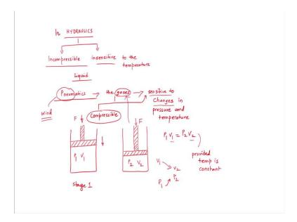
For all practical purposes; we are considering the liquid in hydraulics as incompressible and it is insensitive to the changes in the temperature. Fundamentally, in hydraulics, we are considering the liquid as incompressible and insensitive to the temperature.
