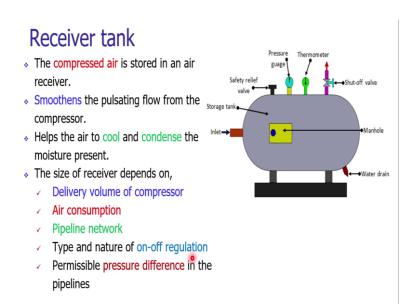
Well, first look at the receiver tank. A schematic of a typical tank is shown on the screen. It is a closed container, it is a sealed container and it has various mountings. It has the inlet and the outlet which has various mounting such as the relief valves, that is the safety relief valve. Pressure gauge to continuously monitor the pressure of the tank. There is a thermometer which is used to monitor the temperature of the compressed air which is stored inside the tank.
