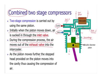
Now, the arrangement of the combined two stage compressor is there on your screen. In this case we are having two pistons. The diameter of the pistons is different. This is the main piston and it has a secondary piston as well. The diameter of the secondary piston is lower than the main piston and to accommodate the secondary piston, a secondary cylinder is also there which is having diameter lesser than the primary cylinder.
