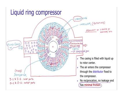
Now, let us study the next positive displacement compressor that is the liquid ring compressor. The technology is very interesting and the reason is very important. In reciprocating type of the compressor, we have seen that there are many mechanical elements and they are sliding. Due to the sliding, there is a friction, due to the friction there is wear and tear of the mechanical parts and due to the wear and tear of the mechanical parts there will be gaps.
