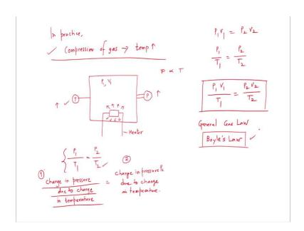
As V 1 is reducing to V 2, the P 1 will increase to P 2. In practice we always experience that the compression of gas is leading to or it is resulting in increasing temperature. Let us consider we are having a closed container, it is a sealed one and inside the sealed container there is a certain amount of gas is present. Volume of the gas is V 1 and it is having pressure P 1 and this container is also having an element which is radiating the heat. It is a heating element basically
