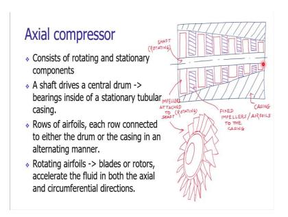
The next type of dynamic compressor is the axial compressor. The axial compressor is widely used. It has the rotating and stationary components. The typical construction of an axial compressor can be seen on your screen. It has a casing, the casing is housing a shaft, the shaft is supported in the bearings which are there in the casing. The shaft is being rotated by an electric motor.
