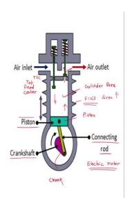
Piston compressors are widely used in pneumatic systems. A single cylinder compressor unit is shown which is generating the compressed air. The construction is very simple, there is a cylinder bore which is having the piston arrangement. The piston is connected to the connecting rod which is connected to a crank.
