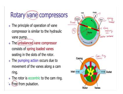
We can utilize the vanes, very similar to the vane pump which we have seen in our the hydraulic pumps section. We can have slots in a rotor and this rotor disc is eccentrically assembled with a stator container. This is the stator container. There is eccentricity between the axis of the rotor and the axis of the stator or the casing. The casing is fixed, it is not moving, it is stationary.
