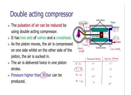
To increase the efficiency of the single acting cylinder, we can also utilize a double acting cylinder. In a single pulse or in a single reciprocatory motion we can generate 2 times of the
