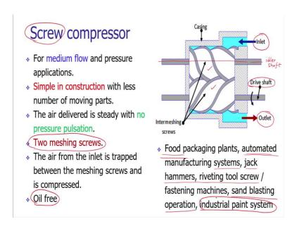
We can also have a arrangement with meshed screws. We are using two meshing screws, a compressor with the screws is shown; that typical arrangement can be seen on the screen. These are the two intermeshing screws and one screw, this screw is on a idler shaft and the other screw is on the drive shaft. The drive shaft is operated, it is governed by the electric prime mover.
