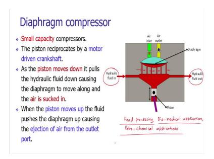
We are having one more interesting configuration based upon the reciprocation motion of the piston and that is the diaphragm compressor. The construction of the diaphragm compressor can be seen on your screen. It has the typical piston cylinder arrangement. This is the piston; there is a connecting rod, crank and crankshaft. The piston is reciprocating and it is driving the hydraulic fluid here.
