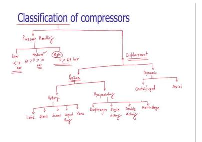
We can classify the pneumatic compressors based on two factors. The first factor is the pressure handling capacity, pressure handling. Here we can have the low pressure compressors, medium pressure compressors and the high pressure compressors. When a compressor is generating a pressure less than 10 bar, it is called the low pressure compressor.
