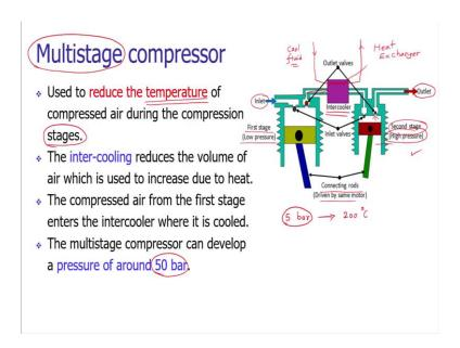
Well, in general the single acting cylinders to generate a pressure of about 5 bar, the temperature may go up to 200 degree Celsius. There is a huge increase in the temperature during the process of compression. To solve this problem and to increase the energy efficiency of these devices, we can go for the multistage compressing. We can use the intercoolers to enhance the efficiency of these systems.
