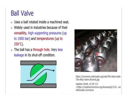
Some steel balls which are machined are shown. This is the circular passage which is machined inside the spherical balls. And, these spherical balls are having the protrusion at the top and at the bottom which is used to get hold inside the lever and the stem arrangement.
