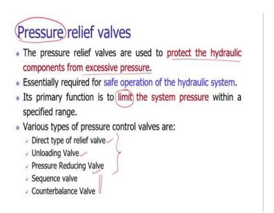
During the hydraulic circuit operations, we need to control the direction of the movement of the fluid as well as we need to control the flow rate of the fluid. In addition to these two important factors we have to control the pressure inside the system. If the pressure of the system is excessively high then that will damage the entire system. There may be catastrophic failure of the hydraulic system, there may be bursting of the system.
