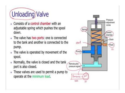
The second type of pressure control valve is the unloading valve. The unloading valve operation is very much similar to the DCV, that we have seen in our previous lecture. In one of the direct control valve we have seen that a pilot pressure can be utilized to use or to convert the direction controlled valve as the unloading valve.
