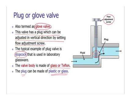
The plug or the glove valve, the plug valve is also called as the glove valve. It is having a plug which is nothing, but a tapered cylindrical component. This tapered component or part is placed in between the passage of the fluid flow. The position of the plug inside the fluid flow
