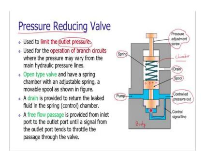
The next pressure relief valve is the pressure reducing valve and the purpose of this valve is to limit the outlet pressure inside the system. By controlling the outlet pressure, we can safeguard the hydraulic system. The typical pressure reducing valve is on your screen; it has the body, the body is having a chamber. The chamber is housing the spool; the spool is being maintained by the spring.
