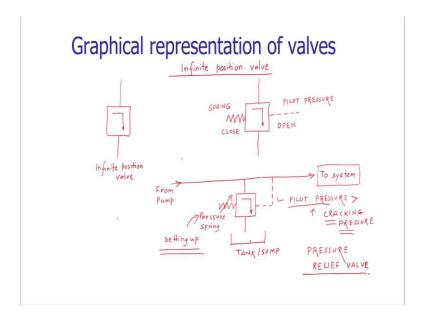
Now, let us see how can we represent the in finite position valve. Infinite position valve is nothing but a valve which is providing a number of position. In general as we have seen that the valves are providing only 2 or 3 the finite number of position, in this case it is providing the infinite number of position so we have to just operate the valve, we have to operate the stem of the valve and we can have a variety of positions.
