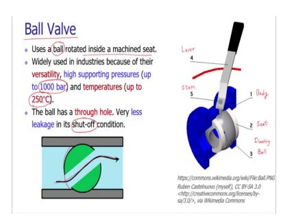
The next type of valve is the ball valve; it is very widely used in the industry. Here we are using a ball which is rotated inside a machined seat. The typical construction of the ball valve can be seen on the screen. It is having the body of the ball valve. There is a seat and that seat is housing the ball, the ball is the floating ball, ball is floating and the ball is having the passage as well.
