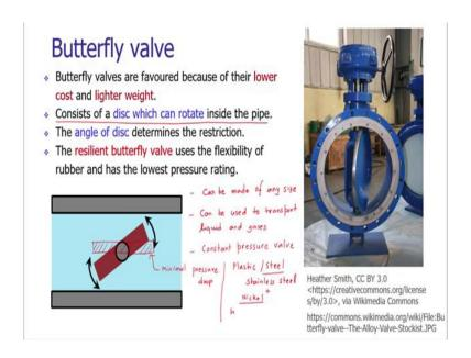
The next type of valve is the butterfly valve. In the construction of the butterfly valve we are using a disc which can rotate inside the pipe, you can see the construction of a butterfly valve. This is the body of the butterfly valve and inside that we are having the disc. As we change the orientation of the disc, we can easily control the orifice, we can easily control the area of passage of fluid flow inside the pipe.
