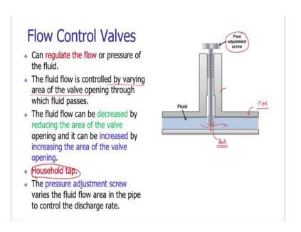
A very basic and simple example of the flow control valve is our household tap. A schematic of a household tap is shown. It is having the pipe through which the fluid is passing and this pipe is fitted with a flow control valve. The flow control valve is having a flow adjustment screw and that flow adjustment screw is having a ball. By rotating the flow adjustment screw we can change, we can vary the orifice area.
