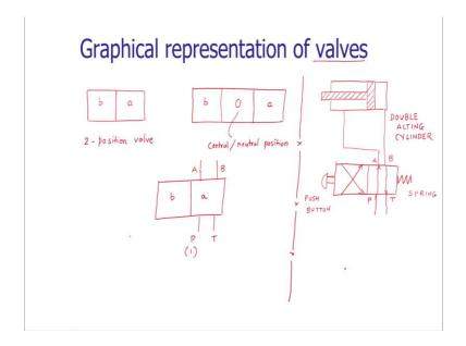
Now, let us study how to represent a typical valve. A valve is represented by a square for each of its switching positions. A typical two position valve can be represented by using 2 squares, now let us draw the 2 squares. This is position b and position a. This is 2-position valve. We can have a 3-position valve as well for that purpose we may need to utilize 3 squares.
