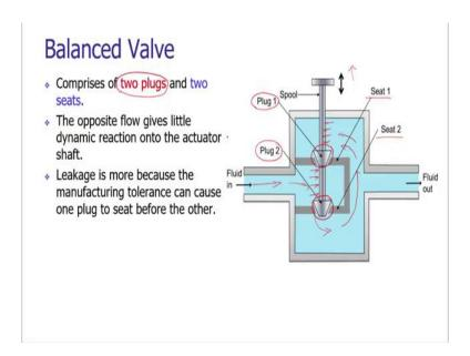
The next type of valve is the balanced valve; the balanced valve is having two plugs. If there is only one plug and one stem arrangement, there may be chances of having the excessive thrust on the stem body.
