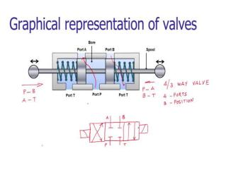
One more example, we will study for the representation of the valves. On our screen, we can see a 4/3 way valve. We have seen the meaning of the 4/3 way valve in our previous class. It is having 4-ports, there are 4-ports and 3-positions.
