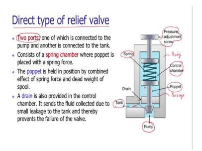
The direct type of relief valve is having two ports. The first port is the pump port at which we are applying the pressurized fluid and the second port is the tank port. These type of relief valves are put inside the hydraulic circuit. When the pressurized fluid which is coming inside the valve if that, pressurized fluid is having pressure more than the specified pressure or the pre-determined pressure then the valve will get actuated.
