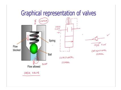
Let us draw the graphical representation of the check valve. Very useful element of hydraulic power pack that is check valve. We have seen the working of the check valve in our previous lecture itself. The check valve is having a ball and a spring arrangement and it is not allowing the fluid in one of the directions, but when the applied pressure is more than the cracking pressure of the spring, then the fluid will be allowed to pass from the other direction.
