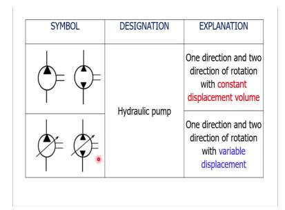
The hydraulic pump is basically designated by using a circle and that circle is having a filled in triangle. The triangle in this format which is filled in that is designating the hydraulic pump.
