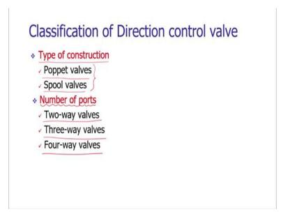
The direction control values can be classified based on many factors, many parameters. The first factor is the type of construction. We are having two types of values which are used in the industry, these are poppet values and spool values.
