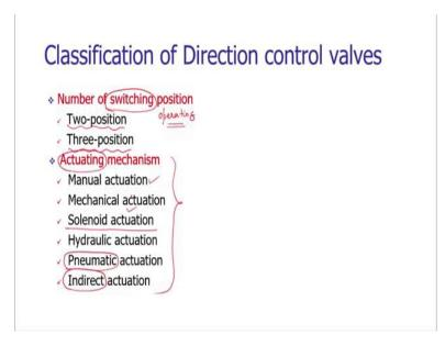
The control valves are also classified based upon the switching position or the operating position. As we have seen in the previous slide for actuation of a single acting cylinder, we need to have the two-position. In first position the fluid is passing at the top side of the piston and the second position the fluid should pass at the bottom side of the piston.
