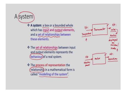
The set of relationship between the input and the output represents the behaviour of the real system. When this relationship is represented in mathematical form, then that process is called the modelling of the system. A simple example of a system is a
