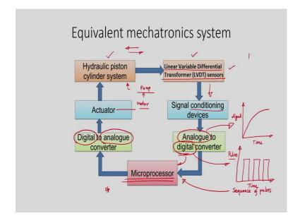
Now, representing all these elements as a block diagram, we have taken the hydraulic piston cylinder system, then we have to select a suitable sensor. In this case, LVDT is considered, which is a linear variable differential transformer. It is contact based displacement sensor.
