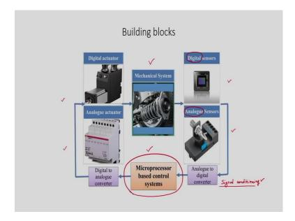
In an arrangement showing the building blocks of an automated system, a mechanical system which is basically being controlled by a microprocessor based control system can be seen. This microprocessor based control system gets inputs from various sensors, which may be digital sensors or analogue sensors. These sensors are further giving signals to signal conditioning devices.
