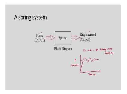
The block diagram of a typical spring system can be seen on the above figure. It is known that, a spring has a force and a displacement and it follows the principle of operation as F=Kx. So, this relation would be true in the case of steady state condition.
