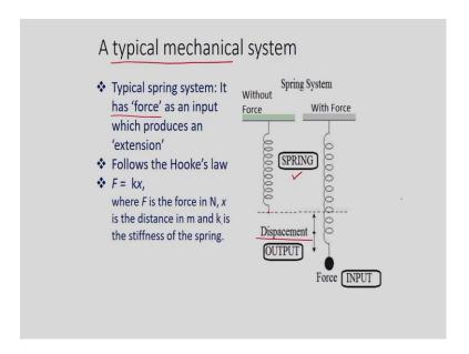
One more example of the term system is a typical mechanical system and that typical mechanical system is a spring. The spring is widely used in variety of engineering applications. The most important or the most common application of spring is in suspension of automotive. The springs comes in a variety of types such as; compression
