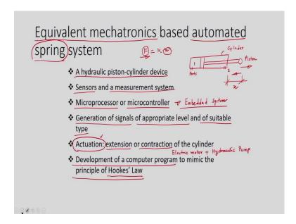
The next building block is generation of signals of appropriate level and of suitable type. Then comes actuation, which is nothing but the extension on or the contraction of the cylinder. This extension or contraction of the cylinder would be done by using pressurized hydraulic fluid.
