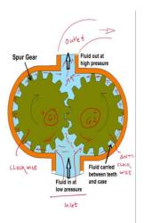
Now, let us look at an interesting configuration of the gear pump that is external gear pump. On our screen you can see there are two spur gears which are meshed together. This is a gear number 1 and we are having the another gear that is a gear number 2. These two gears are meshed and they are assembled in a casing. The casing is having two ports.
