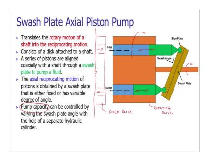
We are having a fixed block here and there is inlet. So, this is the fixed block. Fixed block has the inlet port as well as the outlet port. This is a rotating block. We are giving the rotary motion to the rotating block by using a prime mover.
