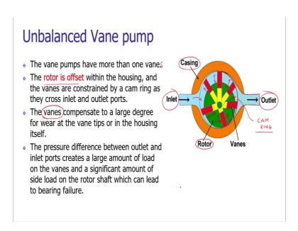
On our screen we can see a configuration of vane pump and it is called as unbalanced vane pump. We can notice the construction. As the cylindrical casing which is having a rotating element that we called rotor. The rotor has radial slots and these radial slots are housing the vanes.
