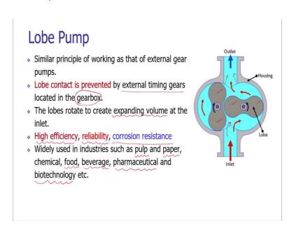
The next variant is the lobe pump. It is you can say the modification of the external gear pump itself. Instead of having many number of gear teeth, the gear teeth profile can be changed into a lobe ship kind of thing. Instead of having many number of teeth we are having only 2 teeth.
