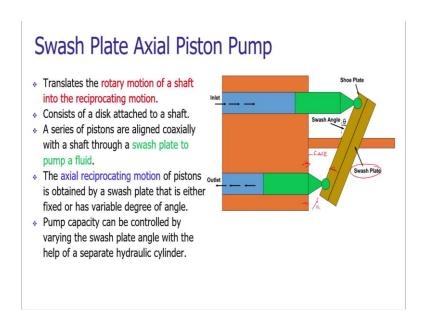
Here a swash plate is used instead of having the bent axis, we are using a plate. The plate is inclined. The plate is not parallel to the surface of the cylinder block. It is inclined to the face of the block. This is the face the block and this swash plate is making angle  $\Theta$ . This swash plate is connected to a shoe plate. The assembly of the shoe plate and the swash plate is mounted on the rod.
