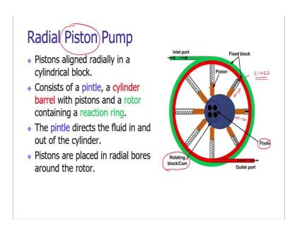
Now, instead of having the axial reciprocatory motion we can also have the radial reciprocatory motion of the pistons. These kind of configuration is called as radial piston pump. The diagram or the schematic can be seen on our screen, which is having a pintle. Pintle is mechanical element which is holding the casing.
