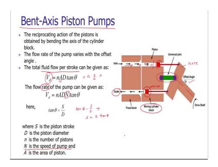
Let us look at the construction and working of the bent axis pump and swash plate type of the piston pump. In the first type that is bent axis piston pumps we are using a moving cylinder block. This moving cylinder block has a number of bores. These bores are thorough bores.
