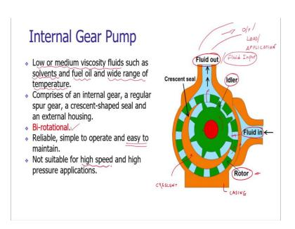
The next variant is internal gear pump. In internal gear pump the construction is little complex. Here we are using a casing. This is the casing of the internal gear pump. There is a rotor. The rotor is having the slots and that slots can get the fluid. There are two ports; fluid in port and the fluid out port.
