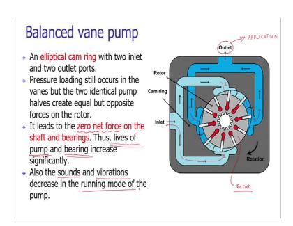
Instead of having one pair of inlet outlet we can have two pairs of inlet outlet. This peculiar arrangement can be seen on our screen. It has the rotor and as usual the rotor is having radial slots with the vanes. The vanes are spring loaded.
