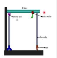
The next version is the gantry crane. It is very similar to the bridge crane itself, but the handling capacity of the gantry crane is lesser than the bridge crane. In gantry crane, we are also using a bridge which is supported at one end on the runway and a rail which is hosted on a support column. The other end of the bridge is supported by a gantry leg. And the gantry leg is moving over a rail.
