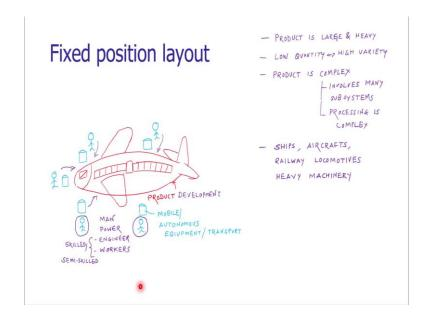
But you consider in certain cases we are having only one product, one system that to be developed. Consider case of aeroplane manufacturing or ship manufacturing, or we can have an example of the railway locomotive manufacturing or heavy machinery. For such applications which are very heavy, very bulky which are difficult to handle very difficult to move from one shop to the other shop.
