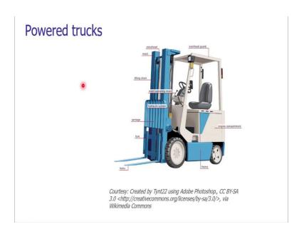
As per as the automation are concerned, we are using the power trucks. Though they are manually operated, but these entities are very much useful in semi-automated industry. Where we are talking about material handling in process layout or in fixed position layout to handle the bulkier component say dies and molds or the tools or the raw material, we need to have an equipment that is the power truck of the forklift truck.
