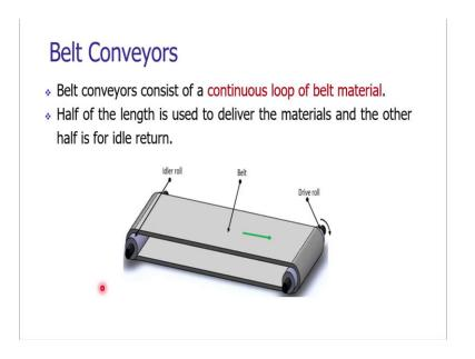
These type of arrangements are basically used to convey dies and molds. The belt conveyors are also very popular and important type. It consist of continuous loop of belt material. So, this is a belt. There is a continuous movement of the belt. The belt is driven by the drive role and there is an idler role. The drive role is being operated by the electric motor. The idler roller is helping to have the sufficient tension in the belt.
