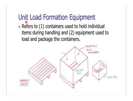
Unit load formation equipment, the unit load formation basically deals with making a container which is holding the individual atoms together, so that we can easily handle them. Let us consider we are having a wooden pallet. The wooden pallet is nothing but a platform of specified size, standard size over which we are putting the finished products say the boxes over each other and with specified number of boxes we are considering that as a unit of a pallet.
