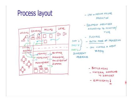
The layout is nothing but arrangement of the equipment or facility inside a factory. In process layout, we are arranging the equipment or the facility based upon the similarity of their utilization. On our screen, you can see a facility related to the tool room. Here we have grouped various equipments based upon their utilization. We can see the sections based upon their utilization, a lathe section, a turning section where we are reducing the diameter of the work pieces.
