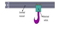
We can have the overhead trolley conveyor. By moving the trolley, we can easily convey the objects with the help of a hook. Over the overhead monorail, we are having a motorized vehicle and it has the hook. We can hand the work part in the hook and then we can easily convey the work part along the length of the overhead monorail.
