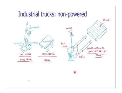
Some simple equipment which are often used on the shop floor and these are the industrial trucks. Some examples are there on your screen. These are non-powered trucks simple two wheel hand truck which is used to transport lighter products. This is the platform over which we are putting the product, and then we can easily convey them. Or
