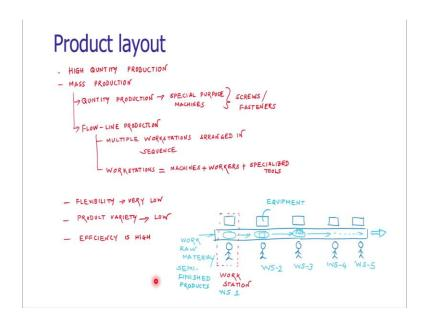
Consider there is a scenario that is of high quantity production. The company is having only one product and we have to produce the product at a high volume at the mass scale. Then mass production as well the production may be a quantity based production. Quantity based production means a manufacturing of screws and fasteners if the companies having the objective to manufacture only one product that is the screw.
