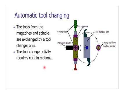
Now, let us see how the tool changing operation is being carried out. In general there are many variants of tool changing operation. Let us look at a simple tool changing operation by using a tool changing arm. In the slide we can see a cutting tool which is mounted on the machine spindle. The spindle axis is perpendicular to the plane of paper i.e. perpendicular to the plane of paper and consider the tool is mounted over here.
