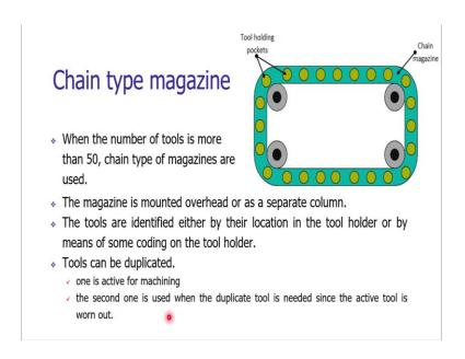
The next type of magazine is chain type magazine. In this arrangement we are using a long chain, which is operated by the sprockets; these sprockets are driven by electric motors. In the chains we are having pool holding pockets, as the chain is moving which is driven by the sprockets we are getting the required indexing of the tools. Based on the required tool a tool changing mechanism will take out the tool from the chain magazine and that will be inserted into the spindle.
