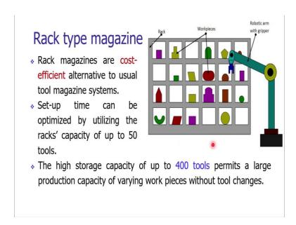
The next type of magazine is rack type of magazine. This is cost efficient, because we can hold more than 300, may be around 400 number of tools in the rack type of magazines. Inside the rack the tools are stored and we need to have a robotic based arrangement to select to get the required tool from the rack and then mount that tool in the spindle of the machine.
