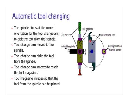
Let us see what are these motions? It is essential that the spindle should stop at correct orientation for the tool change arm to pick up the tool from the spindle. What is the first motion? Proper orientation of the cutting tool in the machine spindle, there is pick up of the tool that to be replaced from the machine spindle.
