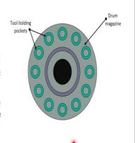
Let us look at the first type of the magazine, that is disc or the drum type magazine. The arrangement is very simple, we are using a disc or a drum and on the surface of the disc or the drum we are generating tool holding pockets. Inside the tool holding pockets the tools are getting mounted. The drum or the disc will be mounted on a spindle on an indexing mechanism, which we have seen in our previous lecture.
