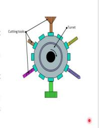
The first and very simple type of tool magazine or tool storage system is tool turret. In the slide, we can see a tool turret, it is a device which can store multiple number of tools, it can be indexed and that indexing mechanisms we have seen in our previous lecture. The tool turrets are generally used on production lathe machines.
