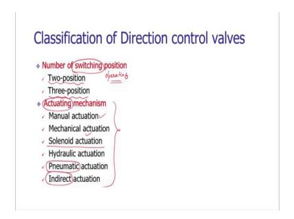
The control valves are also classified based upon the switching position or the operating position. As we have seen in the previous slide for actuation of a single acting cylinder, we need to have the two-position. In first position the fluid is passing at the top side of the piston and the second position the fluid should pass at the bottom side of the piston.
