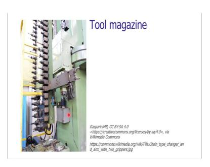
In the slide we can see chain type of magazine; you cannot notice here a variety of tools are mounted. These are the drilling tools, milling tools, the end milling operation tools, cutting operation. The end milling may have a variety of capacity tools, there is a duplication of tool as well. This is the tool changing mechanism. This tool changing mechanism is having an arm, the both the ends of the arm are both the ends of the arm are utilized for tool changing operation.
