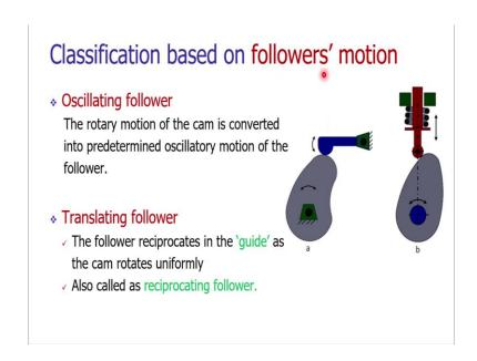
The side thrust will be reduced in spherical face based follower. Followers are also classified based upon the motion. We can have either the oscillating motion of the
