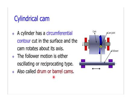
The next variant is cylindrical cam. In cylindrical cam, the cam is in the shape of a cylinder. And we are machining a groove on the circumference of the cylinder. The
