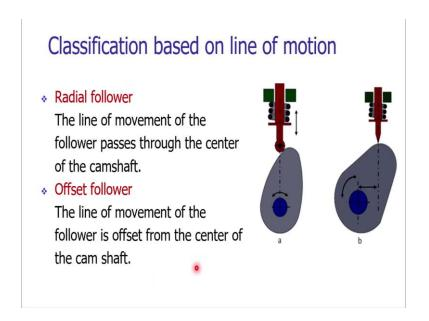
Based on the line of motion as well we can classify. Either we can have the radial followers. The axis of the follower is along the radial direction of the cam itself. The line of movement of the follower passes through the center of the cam shaft. The line of motion is offset with the center of the cam shaft, then we can have the offset follower mechanism.
