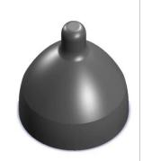
In addition to this two-dimensional cams, we can even have a three-dimensional cam that is called as camoid. It is combination of radial as well as axial cams. It has three-dimensional surface, and it is having two degrees-of-freedom. The cam can be moved along this direction along the radial direction, and it is also moved along this direction as well along the axial direction.
