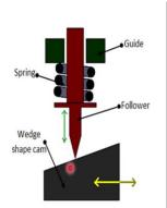
There are various types of cams being used. And we can have the classification such as wedge and the flat cams. In this type of arrangement, we are using a wedge shape cam and the follower is a pointed follower. The shape of the cam is straight; it is not curvilinear. It is a linear cam basically.
