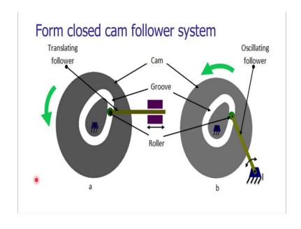
In certain arrangements, we are not applying the external force. We are using the form of the cam itself as a restriction, as an arrangement that will be utilised to ensure the contact of the follower with the cam. For this purpose, we can generate various grooves inside the cam plate itself. And in that grooves, the cam joints are engaged to the cam itself. This groove is ensuring that there is a continuous contact of the follower with the cam itself.
