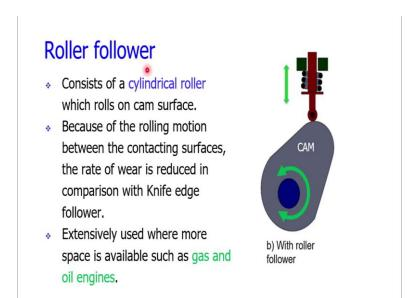
In roller followers, there is rolling friction, rolling motion which is reducing the wear and tear. That is why this roller follower based cams are widely used in gas and oil engines.
