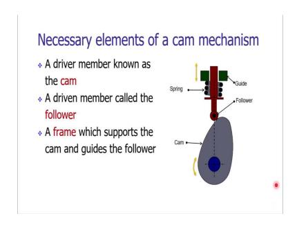
On our screen, you can see a cam as I mentioned right now. We are having a disc. Disc is not in circular shape. It is mounted on a shaft, and that shaft is connected to the electrical drive. There is a follower. That follower is in direct contact with the cam. As the cam is rotating about its axis, it is driving the follower in upward direction.
