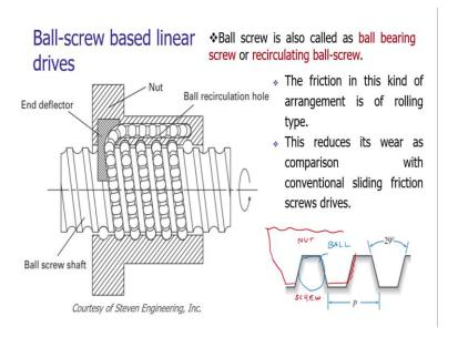
The ball screw based linear drives are also called as ball bearing screw or recirculating ball screw. We know that in a typical screw and nut arrangement, we are having sliding friction. Due to the sliding friction, the efficiency of the typical screw and nut arrangement is low. If we replace that sliding friction with the rolling type of friction, then we can enhance its efficiency. For this purpose, we are using the ball bearing screw concept to get the higher mechanical efficiency.
