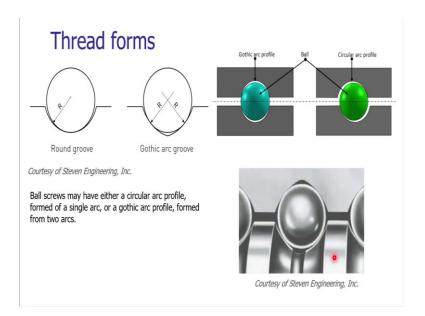
In general, a round groove is developed in this ball screws and in the nut arrangement, but there may be chances of having wear and tear of the screws or the balls. In that case, we may not get the proper contact of the balls with the screws. To have the sufficient contacts or the multiple number of contact points a gothic arc based groove is utilized.
