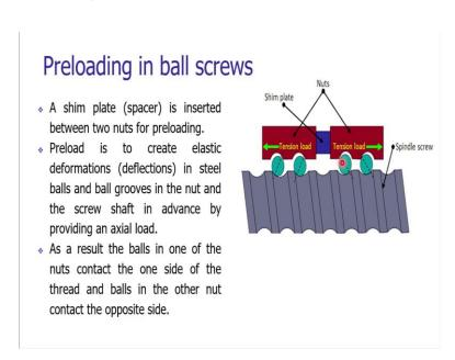
On our screen, we can see a ball which is in contact with the screw and the nut arrangement. Backlash is the problem in ball screws. Due to wear and tear, due to inaccuracies, due to prolonged utilization of the screw and nut arrangement, there may be a backlash, there may be disengagement of the balls with the screw and the nut arrangement.
