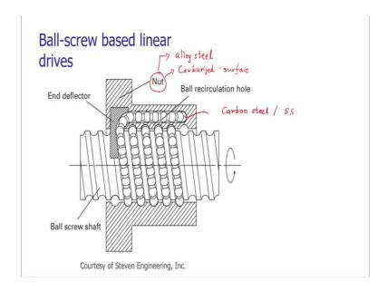
In addition to the screw and the balls, we are having the nut. The nuts are manufactured by using alloy steel and their surface is carburized. The ball circulation system if it is outside is made up of carbon steel or stainless steel.
