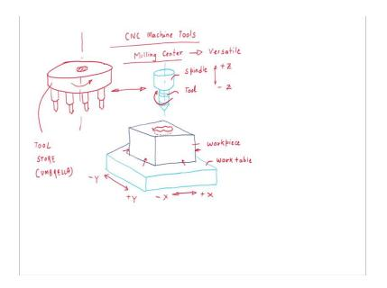
Milling operation is very versatile; very useful in the tool rooms. The CNC milling operation, as we already have seen, is used to develop or used to machine various features, such as slots, pockets, drill holes. The CNC milling operation can also be used to generate complex features. Well, on our screen you can see, a work table on which the workpiece is fixed. It is we are applying the holding force here; we are holding the workpiece on the work table.
