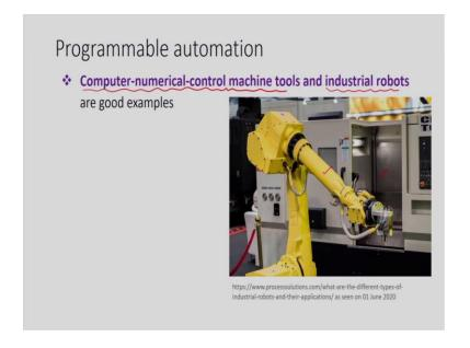
What are the various examples of the programmable automation? Very well-known example is Computer Numerical Control machine tools, CNC machine tools; CNC turning centre or CNC milling centre that we call CNC machining centres. These are the very general and very simple examples of programmable automation. Of course, industrial robots are also good examples of the programmable automation.
