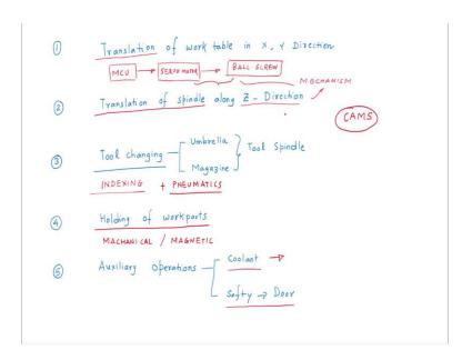
Let us list them down. Firstly, we need the translatory motion; translation of work table in X , Y direction. We also need mechanism for translation of spindle along Z direction. Then, tool changing operation, as we have seen that tool changing would be carried out from the umbrella or magazine to the tool spindle, we need to change the tool.
