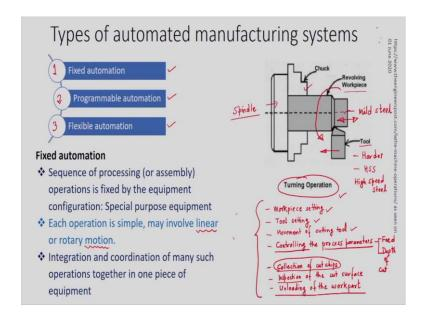
Now, let us see; what are various types of automated manufacturing systems. Basically, there are three types of automated manufacturing systems used in the industry. The first type of automation is fixed automation, the second type of automation is programmable automation and the third type of automation is flexible automation.
