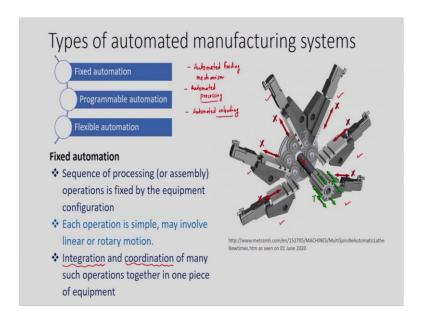
To design such an equipment, we have to integrate all such operations and we have to have an coordination among them. On the right side we can see, you suppose we want to have an specialized equipment, we may need multiple number of tools, and that multiple number of tools are to be mounted on the special slides, that slides are moving with respect to the workpiece.
