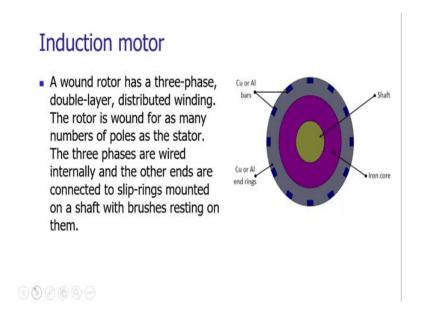
Let us look at what exactly the construction is the rotor is wound with a three-phase double-layer, distributed winding. There is a three-phase electricity supply the layers of the windings are double and they are distributed. The rotor is wound for as many as number of poles as the stator. The winding of the rotor is dependent upon the number of poles of the stator.
