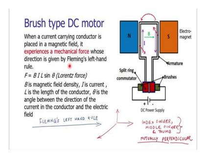
When a current carrying conductor is placed in a magnetic field, it experiences a mechanical force, whose direction is given by the Fleming left-hand rule. To understand the Fleming's left-hand rule, we need to hold the index finger, middle finger and thumb of the left-hand in mutually perpendicular way.
