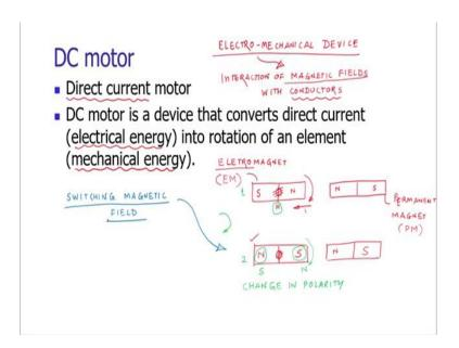
DC motor is Direct Current motor. Direct voltage is applied to this electromechanical device the required mechanical energy is obtained. DC motor basically converts the electrical energy into rotation of a mechanical element.
