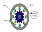
The main difference between the synchronous motor and the induction motor is that the rotor of the synchronous motor travels at the same speed as the rotating magnet.
