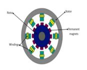
The main difference between the synchronous motor and the induction motor is that the rotor of the synchronous motor travels at the same speed as the rotating magnet.
