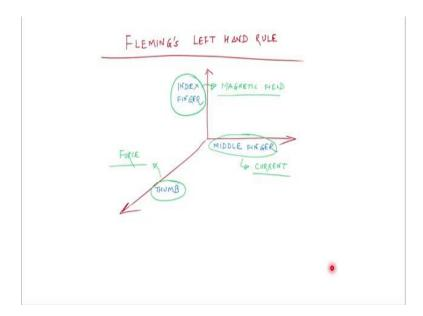
When we are having this arrangement, according to this rule, if the index finger is representing the magnetic field and the current is along the direction of the middle finger, then the force will be in the direction of the thumb. By applying the Fleming's left-hand rule, we can easily find out the moment of the force or the direction of the force along which the conductor is moving.
