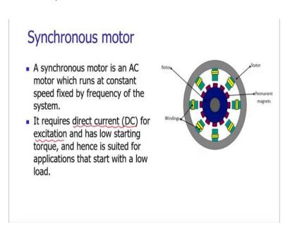
Now, let us look at the first variant of alternating current motor. This is synchronous motor. The synchronous motor is running at a constant speed, which is fixed by the frequency of the system. The synchronous motor requires the direct current for the excitation.
