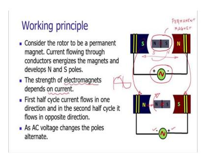
To understand the working principle of AC motor, let us consider the rotor to be a permanent magnet. The rotor is considered a permanent magnet. This is the permanent magnet rotor. The rotor is supported in bearings. And this assembly of the rotor is placed inside an electromagnet.
