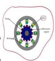
Synchronous motor is a variant of alternating current motor. It has basically two parts that is a stator and the rotor. The construction of the synchronous motor is shown. The stator of the motor comprises of a group of individual wound electromagnets. There are many electromagnets which are having the coils. They are arranged in such a way that they form a cylinder.
