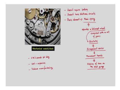
We are using these smart devices regularly. Now, if we look at the mechanical watch, it does not require any battery, it does not have any electronic circuitry as well. All operations are mechanical.
