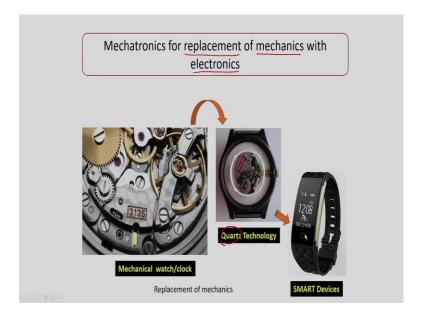
To understand this definition, let us take a simple example. We can see a mechanical watch or a clock in the above figure. There are a lot of components or parts and the construction is very complex. But nowadays, these mechanical watches or the clocks are replaced with electronics clocks or watches. In electronic clock or watches, we are using quartz based technology.
