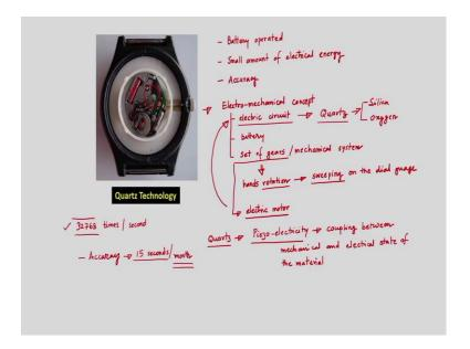
These newer watches are battery operated. In the figure, we can see a typical quartz watch. These watches require a very small amount of electrical energy, as we can notice in our quartz watch, the battery may last long for few months or in certain cases it may go for 1 or 2 years as well.
