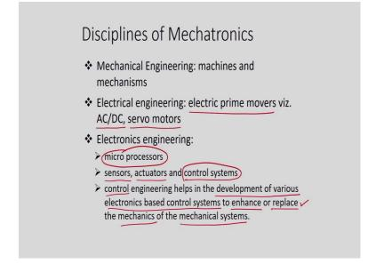
Mechanical engineering contributes in mechatronics by providing various machines and mechanisms. Electrical engineering, provide the prime movers, the electrical energy will be converted into mechanical energy and that mechanical energy will be applied for the intended application, the movement of the various links of the mechanism. For this purpose, we need various motors; AC motor or a DC motor or a servo motor.
