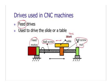
The next application of a drive is feeding the workpiece to the tool. The workpiece is rotating and it is providing the primary motion during the cutting operation, it is providing the cutting velocity, but unless and until the tool is moved with respect to the workpiece, the required size reduction in the workpiece is not obtained.
