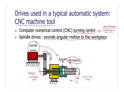
CNC machine tool is the best example to study the utilisation of drives in an automatic system to understand the utilisation of drive. Let us take CNC turning centre. The turning centre is producing axisymmetric components. To produce the axisymmetric components, we should provide the angular motion to the workpiece in relation to the tool motion.
