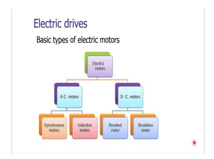
The electric motors are classified into two groups. There are DC motors and AC motor. The DC motors are direct current motors while the AC motors are alternating current motors. In addition to these DC and AC motors, there are other types such as stepper motors. When sensors are used to monitor the revolutions of the motors, these motors are called as the servo motors.
