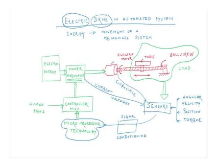
Now, let us define the electrical drive in the context of the automated system. Electrical drive is providing the energy for the controlled moment of the mechanical system.
