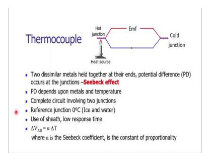
One more important temperature may measurement sensor is thermocouple. It is very much used in the process monitoring and control of manufacturing operations, such as welding. The thermocouple is working based upon the Seebeck effect. What is this Seebeck effect?
