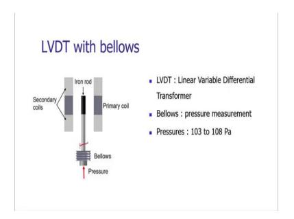
More precise measurement of pressure can be done with bellows when we add the LVDT sensor. On our slide we can see, the LVDT sensor integrated with the bellows. LVDT as we know, it is Linear Variable Differential Transformer. When there is increase in the pressure, the bellows will expand, and as the bellows are expanding the iron rod inside the LVDT sensor will move, it will displace.
