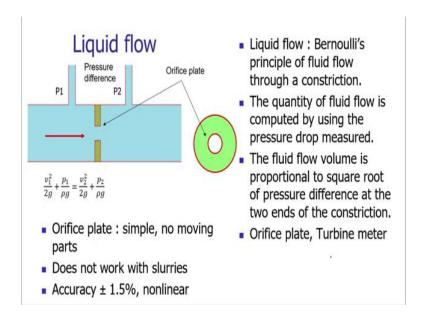
In the industry, we need to measure the flow of various liquids. The liquid may be water; that liquid may be the petroleum products; or chemicals or the liquid may be having certain solid elements that we call the slurries as well.
