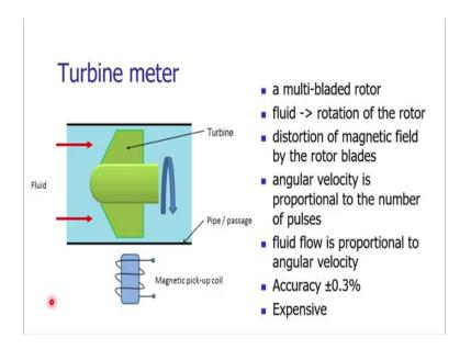
One more popular fluid flow measurement device is turbine meter. The arrangement is very simple. We are having multi bladed rotor. As the fluid is passing over the multi bladed rotor, the rotor will rotate. In the turbine meter, we are having a magnetic pickup coil.
