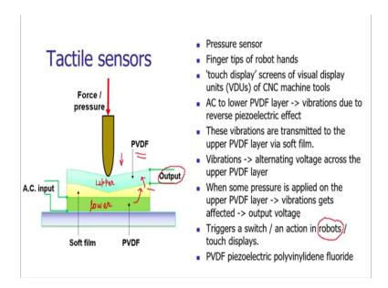
The next interesting sensor is the tactile sensor. It is used to measure the force or pressure. These type of sensors are widely used in the automation purpose and robotics.
