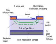
Light irradiates at front surface, anode, while the back surface is cathode. The incidence of light on anode generates a flow of electron across the p-n junction which is the measure of light intensity. Now, let us study the construction of the photo diode. It is constructed on single crystal silicon wafer. The constructional details are shown in the slide. The photo diodes are also called as p-n junction devices.
