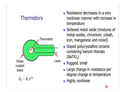
The next temperature measurement sensor is thermistor. In RTDs we have seen, the resistance of the material is increasing with the temperature. In thermistors, the resistance is decreasing in non-linear fashion with the increase in temperature.
