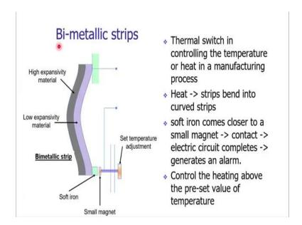
The first sensor is the bi-metallic strips. It is working as a thermal switch to control the temperature or the heat in a manufacturing process. Let us consider an example of a furnace; furnace are used to heat up iron, raw metals and then we are changing its state from solid to liquid. The liquefied metal will be utilized for the casting operation, but the controlled heating of these material is required.
