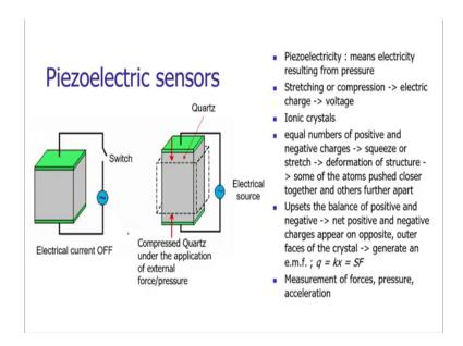
The next type of sensor is piezoelectric sensor. These are very useful and widely used in the industry. What is the meaning of piezoelectricity?
