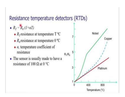
The next temperature measurement sensor is Resistance Temperature Detector. It is very popular and is called as RTDs. The principle is very simple; there are certain materials whose resistance will increase with the application of heat energy. In the slide, we can see the plot of the increase of the temperature with resistance of certain materials such as nickel, copper and platinum. And they do generally follow the equation of increase in resistance as you can see on the screen.
