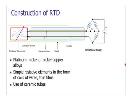
These sensors must be utilized along with a signal processing device. The sensor must be used along with the Wheatstone bridge because the RTDs are providing the change in resistance, but the microprocessor knows the language of voltage. To convert the information from the RTDs that is  $\Delta R$  that will be converted into the  $\Delta V$  by using the Wheatstone bridge.
