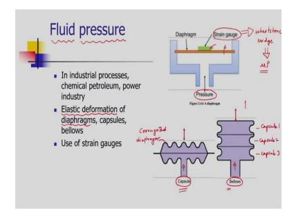
Finally, we will see how to detect the lights by using the photodiodes. Next application; where sensors are required is fluid pressure. In automation we are using variety of fluids; air, gas or it may be water or chemicals or many other liquids. We need to measure the pressure of this fluid for variety of application.
