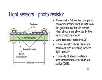
We also require to sense the light in automation. For that purpose, we are using photo resistor. The photo resistor follows the principle of photo conductivity. In photo conductivity, there is generation of mobile carriers when photons are absorbed by semiconductor material. When the light energy will be incident on semiconductor materials, these materials we absorb the photons.
