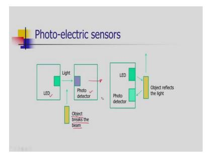
There is another configuration. In this case, the LED and photo detector are put on the same side of the moment of the object. LED is continuously emitting the light, the object reflects the light and the reflection of the object will be detected by the photo detector.
