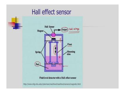
How we can use the Hall effect sensor for controlling or monitoring of fuel, that is a petroleum product. A typical arrangement is shown on the slide. It is having a container, inside the container the fuel is stored. And we need to continuously monitor the level of the fluid.
