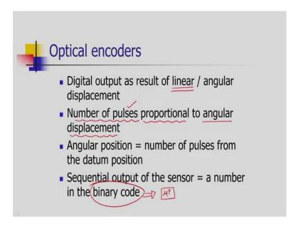
In optical encoders, we are getting digital output as a result of linear or angular displacement. Here linear means that, the same methodology can be used. Instead of rotating signal. we can have a translatory disc: a perforated disc with holes on the disc or a strip. In angular displacement, we are using a disc and in linear encoders, we are using a strip with holes.
