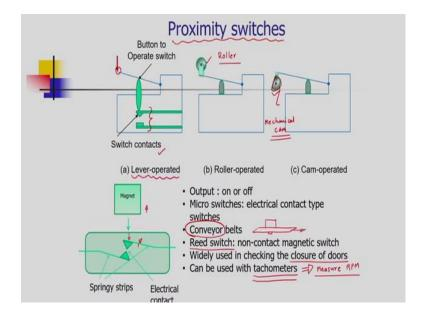
Next group of proximity switches works on the principle of the electrical connection. Now, a simple arrangement, a lever operated arrangement can be seen on the slide. It has switch contacts and these switch contacts are operated by a switch. It is a simple button switch. When we apply a force at the end of the switch, the switch contact will close, there is a contact of these two elements and then there is a flow of current inside the circuit.
