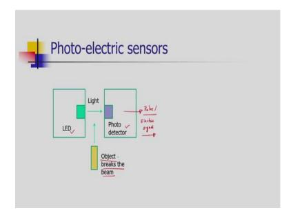
The next group of sensors is photoelectric sensors. In this group, a pair of LED and photo detector is used to detect the passage of light continuously. When an object breaks the beam of light, the passage of light from LED to photo detector generates a pulse. We get a pulse or we get an electrical signal.
