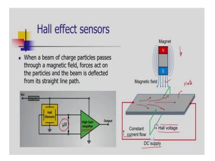
The next type of sensor is Hall effect sensor. The principle of operation is very simple. When a beam of charged particles passes through a magnetic field, forces are acting on the particles. And the beam will get deflected from its straight line path. Due to change in path of the particles, we are getting the voltage across the passage of the original path.
