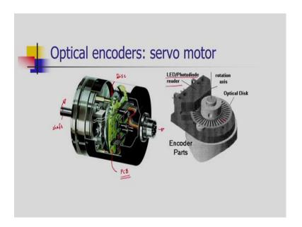
An optical encoder which is mounted can be seen in the slide. A sectional view of a drive is also shown. Inside the drive, a shaft can be seen and the rotation of the shaft is to be measured by using an optical encoder. herein the given figure, an optical encoder disc is shown.
