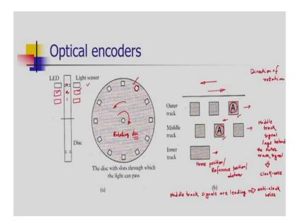
Now, we will see how to measure the motion in angular mode. For this purpose, optical encoders are used. A typical optical encoder can be seen on the slide. It has a rotating disc; this disc is mounted on the element of which we want to measure the angular motion.
