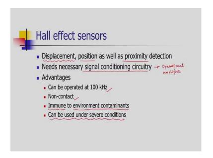
Let us see what are the applications of Hall effect sensors? Hall effect sensors are used for sensing the displacement, position as well as proximity. Of course it needs signal conditioning circuitry, as mentioned the operational amplifiers.
