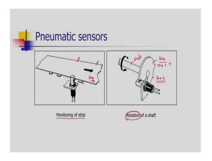
What are its applications? Now, first application we can find in orientation of the products which are moving over the conveyor. Considering a strip which is moving over a conveyor. If by mistake we have kept the strip at certain offset, that may create further problems in production.
