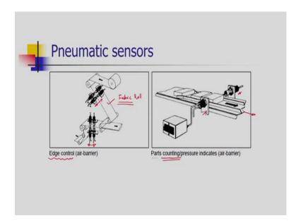
The next operation is to control the edge. Considering textile or a fabric roll and these fabric roll is feeding the fabric for further cutting operation. It is highly essential to have the proper flow of fabric through the system. For that purpose, the edge of the fabric is to be monitor continuously. For that purpose, a set of sensors are mounted. Again, the same principle is applied to monitor continuously the edge of the fabric.
