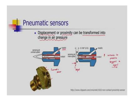
Next sensor is a very useful sensor in automation. it is working with the help of pneumatic energy, compressed air is in general used. It is used to measure the displacement or to detect the proximity of the products or the objects. Here, the principle of operation is that, the displacement will be transformed into the change in air pressure. And that change in air pressure generates the signals, that signals can be utilized for our decision making.
