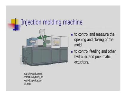
The next example is an injection molding machine, this is used to manufacture plastic components. In injection molding machine, we have molds which are having two parts;, so we should have a precise opening and closing of the molds. For that purpose, we have to control its operation; the molds' inertia and weights are also very high.
