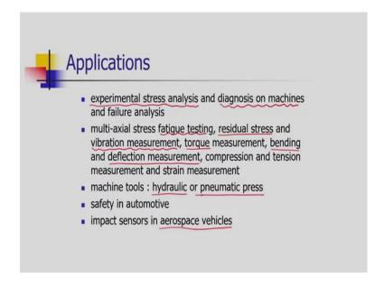
Basically strain gauges are widely used in experimental stress analysis. For stress analysis and for diagnosis of machine tools, strain gauges are widely used, particularly to measure the forces. Moreover for fatigue analysis, fatigue testing, stress analysis, vibration measurement, torque measurement, bending and deflection measurement the strain gauges are used.
