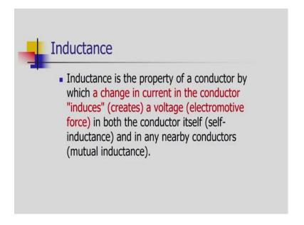
The next electrical property which is helping us to design a sensor is inductance, which is useful to develop a sensor.
