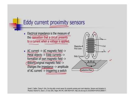
The next proximity sensor is eddy current type proximity sensor and it works on the principle of electrical impedance. Impedance is the measure of the opposition that a circuit presents to a current when voltage is applied. Consider a circuit in which the current is flowing; when the voltage is applied, the circuit will oppose the current. This is called as the electrical impedance.
