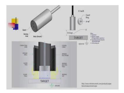
A typical industrial construction of these capacitive sensors are shown. This is the sensing area which is small; however the sensing area is guarded by the guard area, and the guard construction and the sensing construction are enclosed in a body. Capacitive proximity switches are working with target, only condition is that the target should be grounded. When these capacitive sensors are coming closer to the target, it produces the signals.
