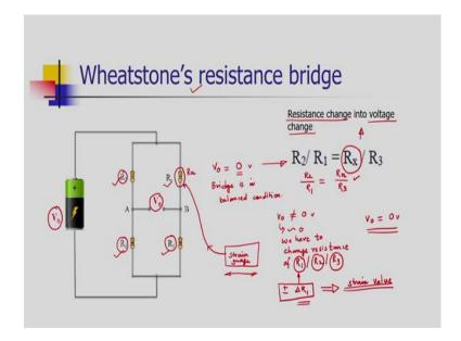
The strain gauge element is providing the passive output. Passive output as is producing the change in resistance; but for microprocessor processing, we need the active element, the voltage change in voltage; a pulse of voltage that is the digital signal that is useful for the microprocessor. For that purpose the resistance change have to be converted into voltage change.
