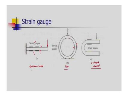
Now, on the screen we can see, how the vibrations are measured. If suppose we are applying a repetitive load at the cantilever beam here, the load is applied intermittently; then the strain gauges which are pasted on the top surface are experiencing tension due to the tension in the fiber of the top surface.
