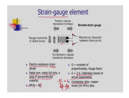
The next important displacement sensor is strain gauge element sensor; it works on the principle of change in resistance when we are giving tension or compression to a mechanical element.
