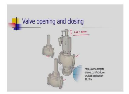
There are very huge size valves which are used for controlling the direction of the fluids, the water. To control the flow of water, these huge types of valves are used. These valves' openings and closing are operated by using an electric motor; when these electric motors are operating, there is movement of its spools.
