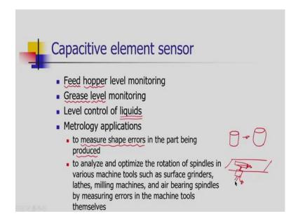
What are the applications of capacitive element sensor? They are used to monitor the feed in hoppers. Hoppers are nothing, but a material handling device through which the commodities inside automated system are fed. Let us consider an injection molding; the hopper is nothing, but a conical flask which is mounted on the injection molding machine, through which we are feeding the granules of the polymers inside the mold area.
