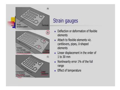
Some more pictures are there, which will clear the idea of the strain gauge. We can see the strain sensitive pattern and the terminals of a typical strain gauge.
