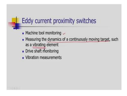
Various applications of the eddy current proximity switches can be seen on the screen; these are used to monitor the machine tool performance. The eddy current proximity switches are very useful to continuously monitor the moving targets and that is the vibrations.
