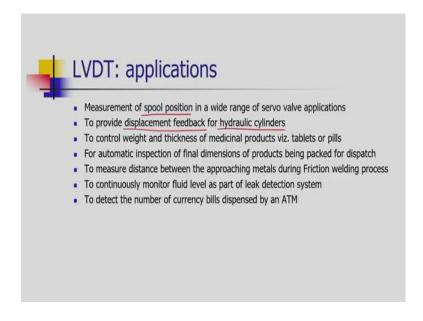
Another application is the spool position measurement or control of spool position. Then displacement feedback in hydraulic cylinders; because hydraulic cylinders are being operated by high pressurized fluid.
