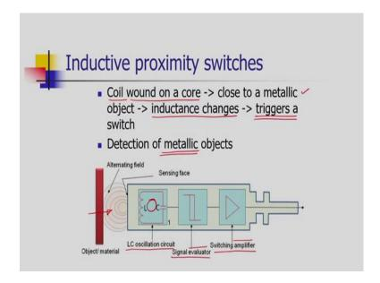
This electrical property is helping us to develop inductive proximity switch. A typical construction is shown on the screen. We are having the LC oscillation circuit, inductance capacitance oscillation circuit; then there is a signal evaluator and then switching amplifier. Evaluator and amplifier are signal processing devices. When inductive proximity switch comes in vicinity of object of material, an alarm is generated.
