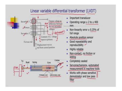
The next important and useful transducer which is used in automation is linear variable differential transformer and it is widely known as LVDTThese kind of sensors are used to measure the displacement between plus or minus 2 mm to say about 400 millimetres; these sensors has non-linearity error of 0.25 percentage.
