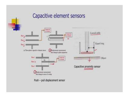
We are taking three plates; plate number 1, plate number 2 and plate number 3. Now the second plate is attached to the element of which we need to measure the displacement.
