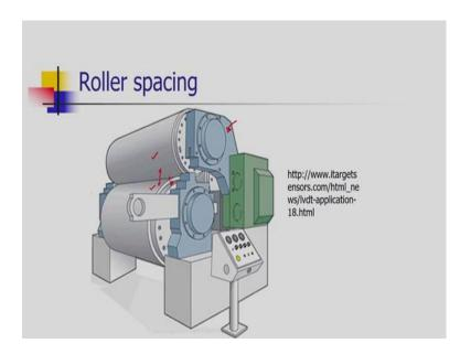
What are various applications of the LCDT sensor? We can see a mill, the mill has two rollers and this mill is used to reduce the thickness of a metal sheet. There is an arrangement here to adjust the spacing between these two rollers. To adjust the spacing between these two rollers, we have to mechanically move the upper roller with respect to the second roller which is at the down side.
