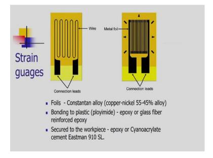
Two more pictures are there on the screen; in the first picture we can see a thin foil and on the thin foil, a wire is wound, which is attached.
