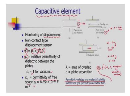
The next sensor is capacitive elements sensor; its advantage is that it is a non-contact type of sensor and used to monitor the displacement.
