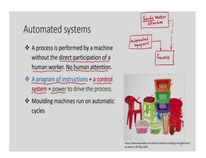
The third manufacturing system is the automated system. In automated system a process is performed by a machine and there is no direct participation of the human being. Thus, at advanced automated system level we can say that there is no human attention even required to carry out the manufacturing operation.
