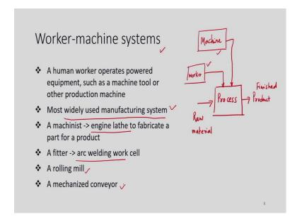
The next type of or category of the manufacturing system is worker machine system. A worker machine system is a human worker or operator using powered equipment such as machine tool or other production machine to carry out the conversion operation. So, we will try to find out a block diagram. We can say that there is a process of conversion of raw material into the finished product, we need the worker and we need the machine as well.
