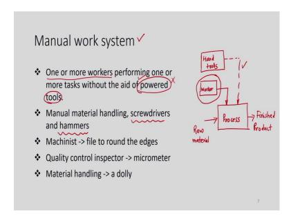
Now, let us see what is the meaning or what is the meaning of manual work system. Manual work system has one or more workers and these one or more workers are carrying out the manufacturing operation with the tools, but the tools are not powered. The simple example is a carpenter.
