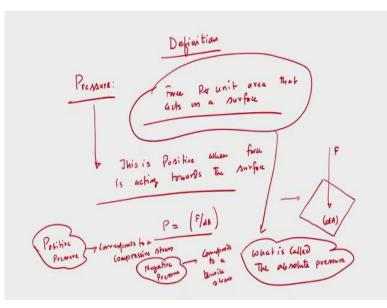
So, we start with the definition of pressure that is what we would like to measure and pressure is one of the important flow parameters we need to measure and in most of the fluid dynamic applications we measure pressure in dynamic condition, that is whenever fluid is flowing in a fluidic pathways, then we measure what is the pressure. Many a times we are interested in to measure pressure in the dynamic conditions.
