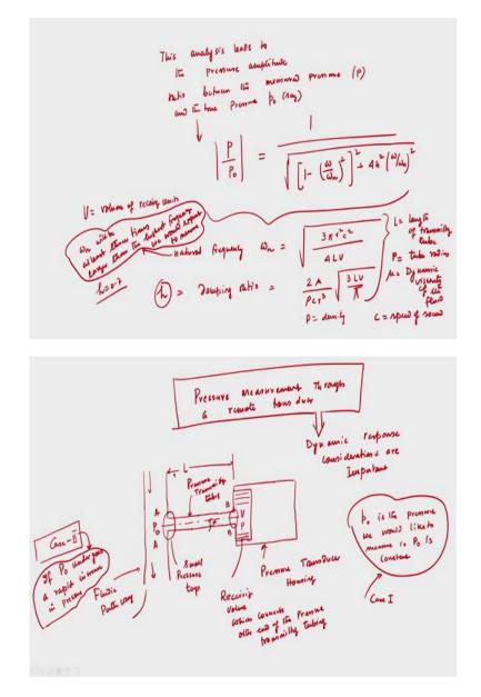
So, this analysis leads to the pressure amplitude ratio between the measured pressure and the true pressure, between the measured pressure say P and the true pressure and the true pressure say P naught say. And that is given by P by P naught mod that equal to 1 by root of under root of 1 minus omega by omega n square total whole square plus 4 h square into omega by omega n square.
