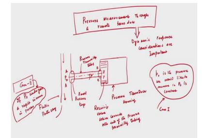
So, pressure measurement through a remote transducer and while we are measuring using, while you are measuring pressure using remote transducer then the dynamic response considerations are become important, considerations are important. Now, we need to know why, why it is important.
