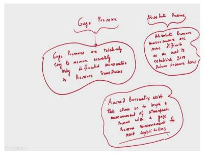
So, gauge pressure that is what we have defined, gauge pressure and we have also defined the absolute pressure, gauge pressures are relatively easy to measure using any differential manometer or pressure transducer, not only that they can be measured more accurately. While, absolute pressures are very difficult to measure. So, I can write, this is very important
