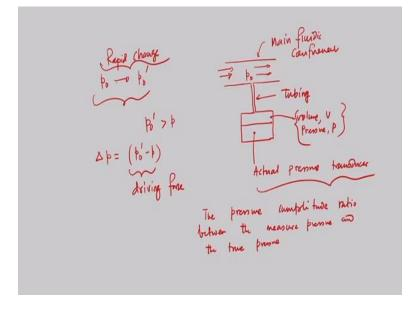
So we have fluidic confinement through which a fluid is flowing and we have taken pressure tapping and this pressure tapping is used to measure pressure and we have seen that this volume is v, pressure is p. So the volume between the inlet and the actual pressure transducer, so this is the actual pressure transducer, so this is actual pressure transducer.
