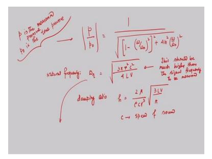
Now because of this phenomenon the pressure amplitude ratio between the measured pressure and the true pressure that we can calculate and if we calculate that is not in the scope of this course, but we can calculate this p by p naught, this expression I used in one of my previous classes that is nothing but 1 upon root of 1 minus omega by omega n square plus 4h square square, their natural frequency omega n, this is the, that is 3 pi r square c square by 4 L into V under root.
