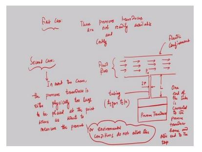
So that means if we now go to the next slide and we can write. So first case we are discussing, then what we can write that this pressure transducer are very costly and as a result of which what is done, this is not the, although this method is suitable but this is not used in practical application.
