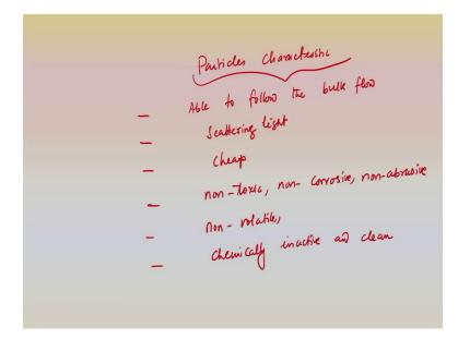
Finally, I would like to discuss, I would like to write, the particles, particles characteristic that means, as I said density of the particles will be more or less equal to the density of the fluid that means, they will have, they will be able to follow the bulk flow, then, I mean, they will be able to scatter light or scattering light, cheap, then non-toxic, non-corrosive, non-abrasive, non-volatile, chemically inactive and clean.
