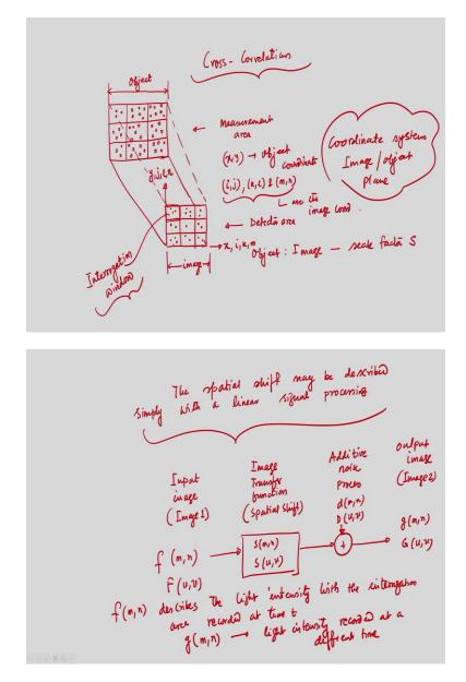
Through a block diagram, the spatial shift, the spatial shift, may be described simply with a linear signal processing. So, if I show, that input image, that is image 1, then image transfer function, spatial shift, additive noise process, output image that is image 2. So, the spatial shift that is what I was telling, the spatial shift of the seeding particle may be observed from one sample to its counterpart in the second camera image, provided the flow is there in the illuminating part.
