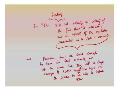
So, the seeding particles and the seeding effect is another important part of this analysis. So, what I said, in PIV analysis it is not actually the velocity of the flow that is measured, but the velocity of the particle that is measured. So, in PIV, it is not actually the velocity of the flow that is measured, but velocity of the particles suspended in the flow is measured and as if the particles are acting like the probe.
