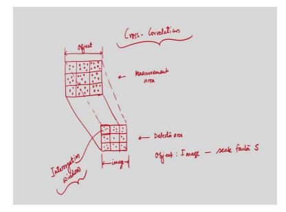
So, in the last lecture, we have discussed about the image capturing technique and from there, from the captured image we need to correlate, so that, we can obtain the velocity of the particle, and if we can predict the velocity of the particle, then from there, we will try to predict the velocity of the fluid, and that is, what is the objective.
