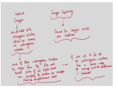
So, if we can recall that we have discussed about the image capturing. So, image capturing and then from image capturing another module will be to processing of the, to process the images which are captured. So, this is another important aspect, if we can recall correctly that in the last class we have discussed that the, you know images, the camera images are divided into rectangular windows and these windows are known as the interrogation windows.
