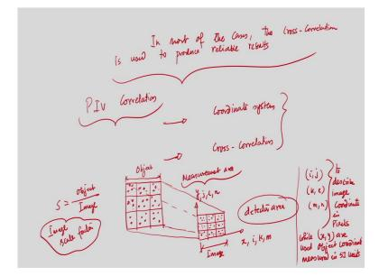
So, I am writing in most of the cases cross-correlation is used to produce reliable results. So, we will discuss the cross-correlation algorithm which is used to produce the trustful result. Now, to discuss about the PIV correlation, first we need to discuss about the coordinate system. And then second, we need to discuss about the cross-correlation. So, what is coordinate system?
