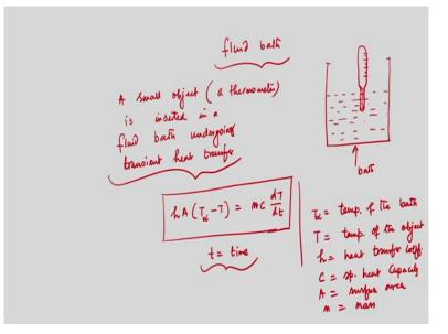
Say we have a fluid bath and this is filled up with 1 fluid and if we use a thermometer, so we can measure the temperature of the liquid of the fluid which is kept in the bath. So, this is bath, so now a small object or thermometer is inserted in a fluid bath undergoing transient heat transfer. That means, if we insert the thermometer, a small object in the fluid bath, then we would like to measure the temperature.
