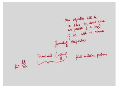
What we can tell that, I am writing that our objective will be to have as small as you know a time as possible, as small a time as possible, that is k is large if we wish to measure fluctuating temperature. So, that means our objective when we are designing a thermometer that is the object, our objective should be to design in such a way that we can correctly capture the fluctuating temperatures.
