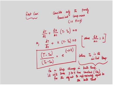
So, as the first case, the first case consider only the purely transient component. That is F equal to 0. Then we can write the equation d capital T by d small t by mc T minus Tm equal to 0 or if we solve this equation I can write dT by d small t plus some constant k into T minus Tm will be equal to 0 where hA by mc is k. Then T minus Tm divided by T naught minus Tm.
