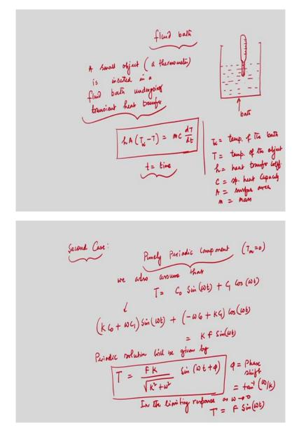
Then, if we try to cross the equation that is what we have written in the previous slide that this equation, then we will get the solution which is given by this. T is equal to F into k by you know k square plus omega square into sine omega t plus phi. So, here the phi, it is equal to phase shift, that is tan inverse omega by k and in the limiting case, so we can write that in the limiting case, a limiting response as omega tends to 0, t will be equal to F sine omega t.
