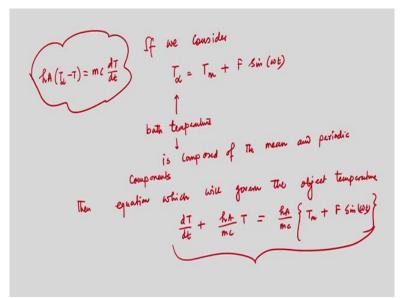
Now, if we so this is the equation. If we consider that T infinity is T mean plus F sine omega t. That is, this is bath temperature and this bath temperature is composed of the mean and periodic component. That means, if the T infinity is TM plus F sine omega t, that is, it is having the mean component as well as the periodic component, then that equation which will govern the object temperature will be, so we had hA T infinity minus T, that is mc dT by small dt.
