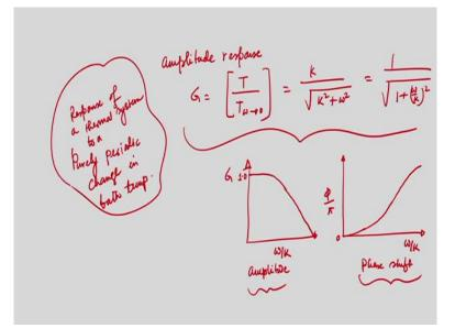
So, now question is what will be the amplitude response and that is G that will be equal to T by t when omega tends to 0 and that is k by root k square plus omega square, that is 1 upon root of 1 plus omega by k the whole square. So, this is the amplitude response. So, this is important because that is what I am not going to discuss, we have learned this in our mathematics course.
