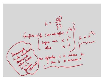
Now, then objective should be to increase k. That means, if we increase r, that means, that is to increase, sorry to decrease r. That is to decrease r. That means, if we reduce r, we can increase k and if k is increased, our objective will be fulfilled. That means, we can measure
