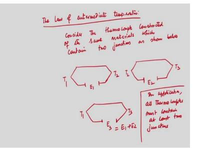
And we have discussed the Thompson effects is usually ignored, because the, I mean the EMF which is produced which will be equal and opposite and they will cancel each other. Peltier effects can be eliminated by considering high input impedance voltage measuring circuits. So, from these three effects we can say that as if a thermometer can be calibrated, thermometer can be created by calibrating the output voltage across the non-junction ends of the wire, if current is very small.
