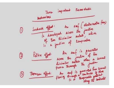
So, now you should know the three important thermoelectric mechanisms and these three important mechanisms are important to describe, to understand the operational principle of the thermocouple and of course, to know by how a thermocouple measures temperature. What are those three important effects? We have studied these effects in our 10 plus 2 level, you know, physics course, so but today just I am trying to recapitulate all those.
