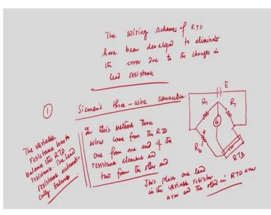
So, we can say that the wiring scheme of RTD, schemes of RTD have been developed to eliminate the error due to the changes in lead resistance. So, that means we have understood that the RTD which you need to place in the Wheatstone bridge through leads, leads will definitely have resistance but depending upon the ambient conditions of the wires of the RTD and bridge, lead will have different temperature and this will lead to error in the measurement techniques.
