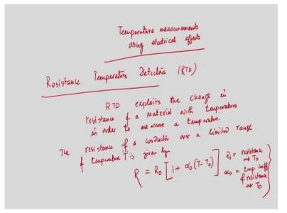
So to start with, we will see that, that is temperature measurement using electrical effects, so that is what would like to know that and to know the measurement technique of temperature using electrical effect, we should discuss the resistance temperature detectors, so, that is resistance temperature detectors or RTD in short. So, the resistance temperature detectors basically they exploit the change in resistance of the material with temperature to detect the temperature difference.
