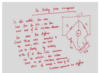
And then we have also discussed about the four-wire scheme and we have seen how using the scheme we can ignore the resistance rather the lead resistance, the error due to the lead registers and finally, we have discussed about the floating point arrangement, also we have discussed that how we can check on the resistance measurement, where I mean resistance due to the leads can be, I mean can be compensated.
