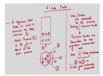
So, the 4 hole probe, 4 hole probe, so this 4 hole probe, 4 hole probe is used to measure flow parameters that is a static pressure, stagnation pressure and also, we can measure the velocity components. So, today we will see that using this 4 hole probe, how we can measure the velocity components. That is very important in, you know in different areas of fluid mechanics research, in particular where I would like to measure, you know excel flow machines or in different other turbo medicines.
